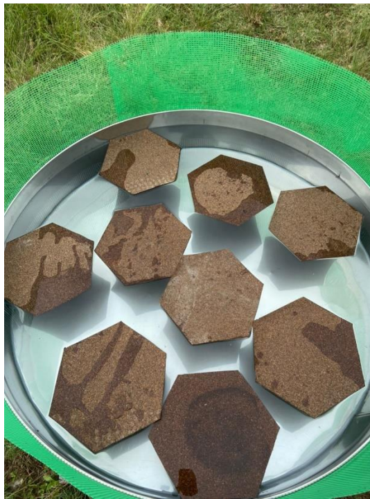
Figure 3.2 Hexagonal cork sheet in pan evaporation
