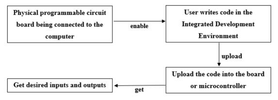
Figure 4: Arduino Development Process
