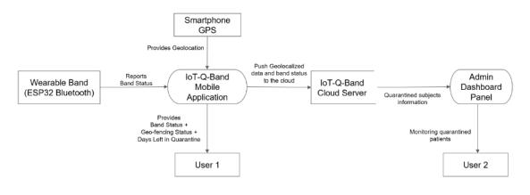
Figure 2 : IoT Q-Band Dataflow
