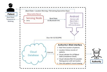
Figure 1 : IoT Q-Band System Architecture
