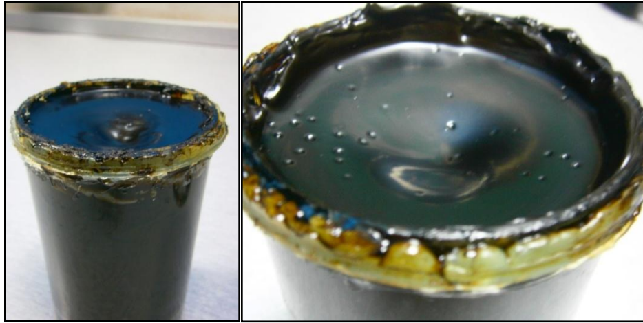
Figure 31: Slow cooling rate (Right) and Fast cooling rate (Left)
