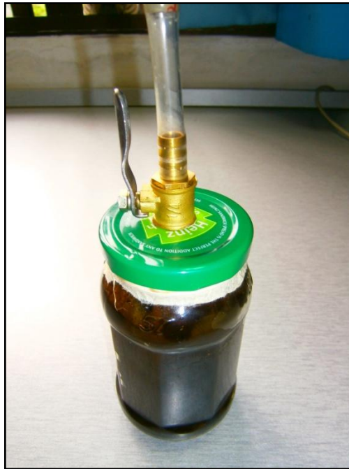
Figure 23: High pressure resistant crude tank
