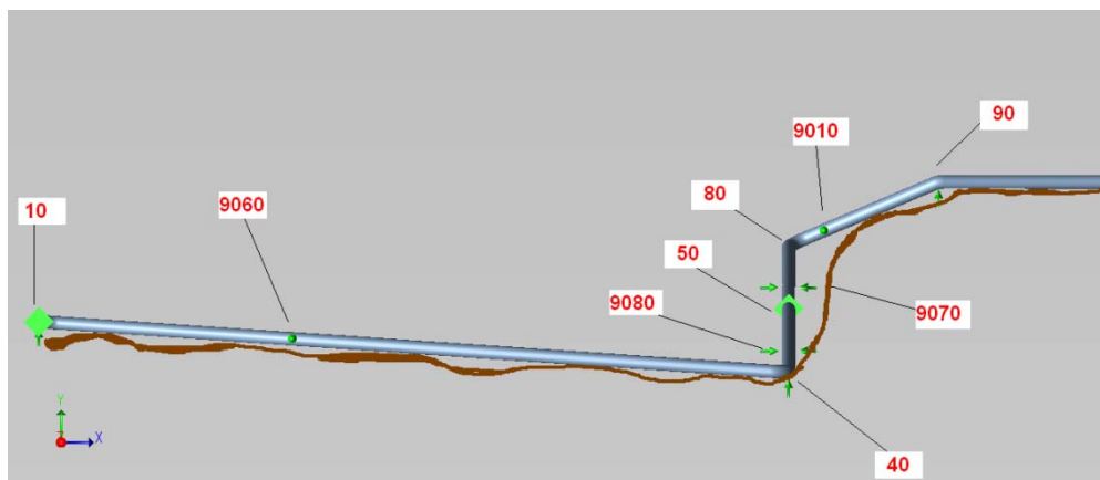
Figure 19: Slide-down shaped topography applied on the pipeline routing (Brown line indicates the seabed topography)
