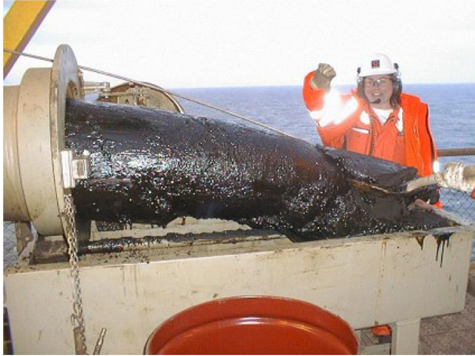
Figure 1: Part of wax plug retrieved from Statfjord B (Sept 01)- taken from “Pigging of Pipes with High Wax Content” by Alf Tordal (2006)
