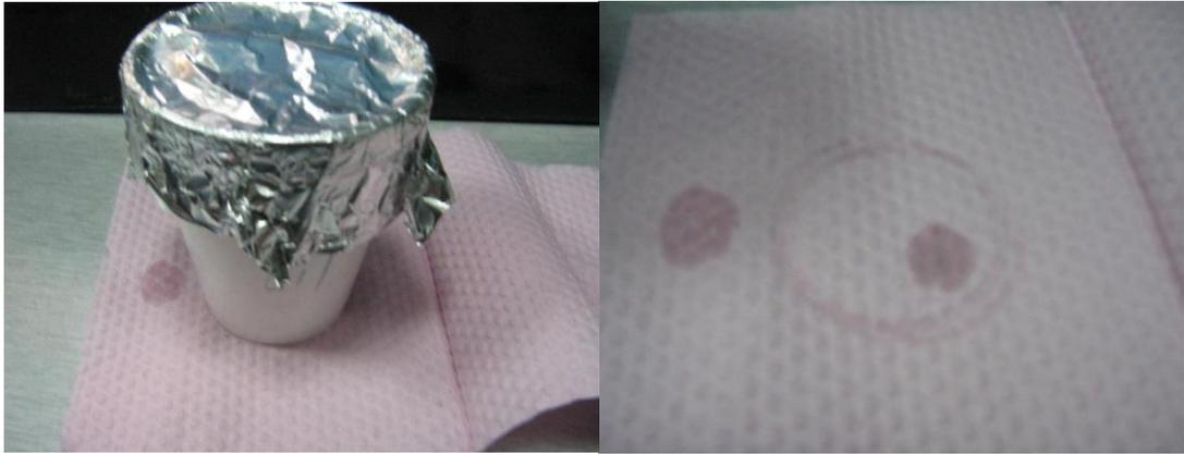
Figure 4.9: Oil marks on tissue paper, indicating cooking oil penetrating through the PS cup.
