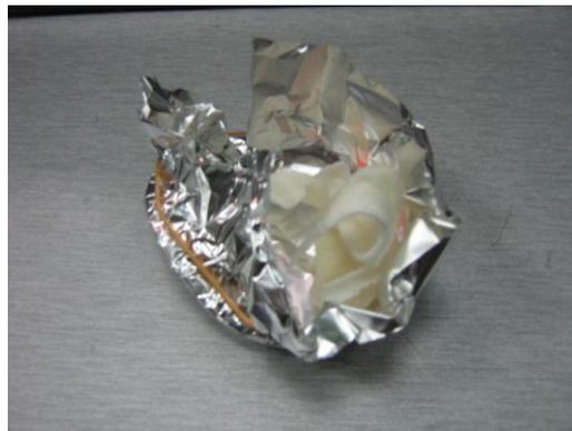
Figure 4.11: Ruptured PS cup at 125°C.
