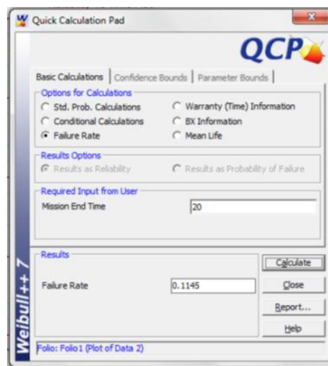
Figure 13: QCP for Failure Rate of Data Set II
