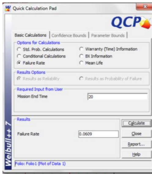
Figure 9: QCP for Failure Rate of data Set I.
