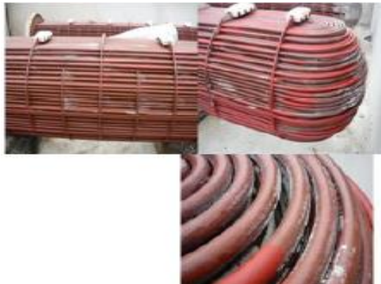
Figure 4.13: Peeled off coating in some areas due to water jetting [12]
