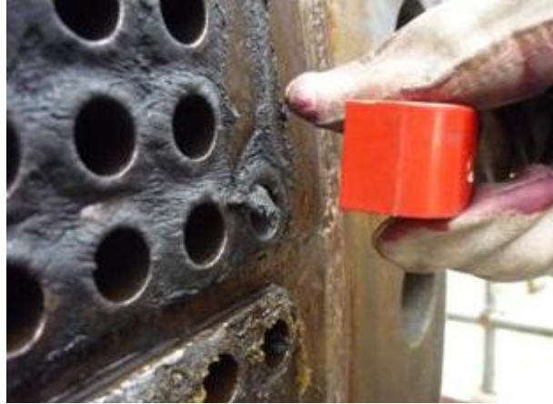
Figure 4.19: Magnetic test carried out at deposited surface [12]
