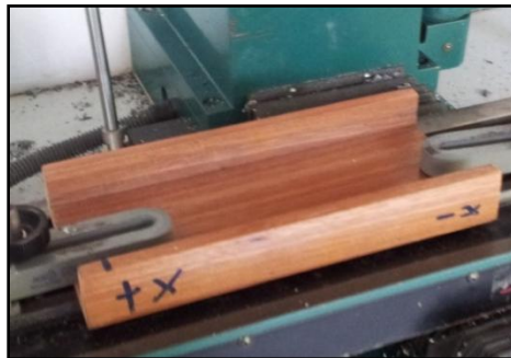
Figures 8 : Jig to support and hold the sample
