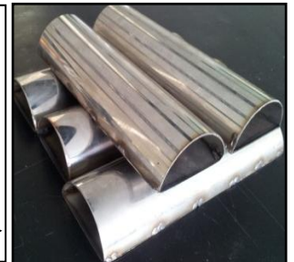
Figure 19 : Molds obtained by halving stainless steel pipes and spot weld with plate at bottom
