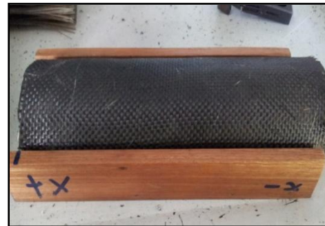
Figures 8 : Jig to support and hold the sample
