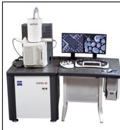
Figure 17: An example of a FESEM machine
