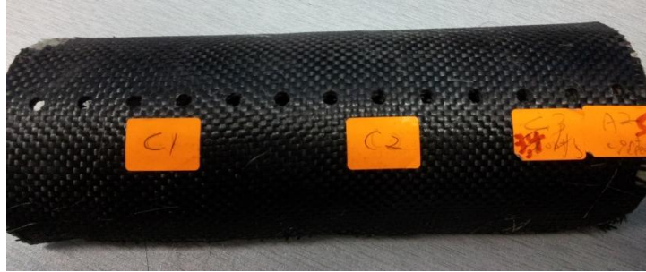
Figure 22: Holes drilled in one of the fabricated samples
