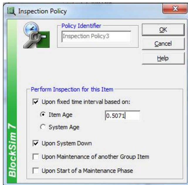
Figure 16: Inspection policy setting window in BlockSim
