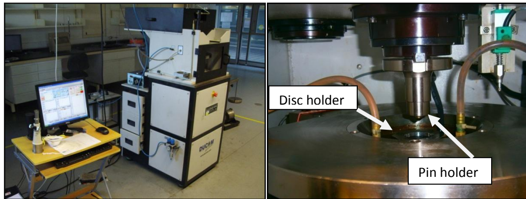
Figure 3: (a) Ducom TR-701-M6 Multi Specimen Tester machine and (b) pin and disc holder.
