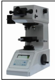
Figure 4: Vickers hardness test instrument; Model HV-1000A Micro Hardness Tester
