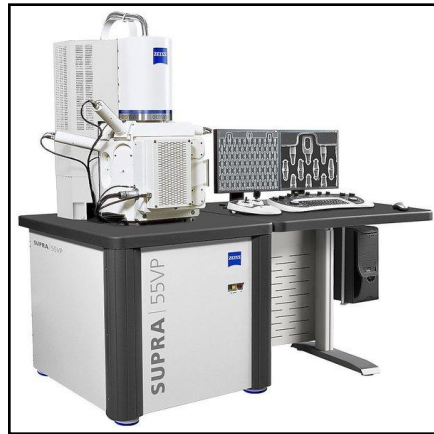
Figure 5: FESEM instrument; Carl Zeiss AG - SUPRA 55VP
