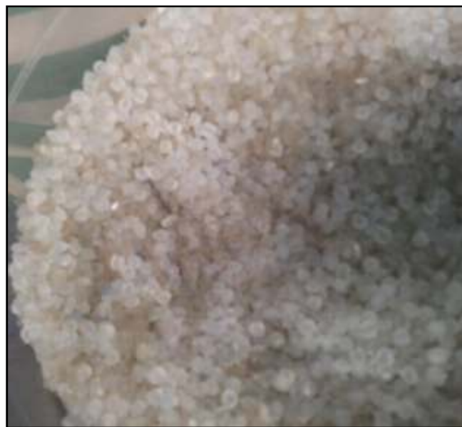
Figure 1.3: Mixture of PP/PET/PP-MA with ratio 70/30/5 wt%.
