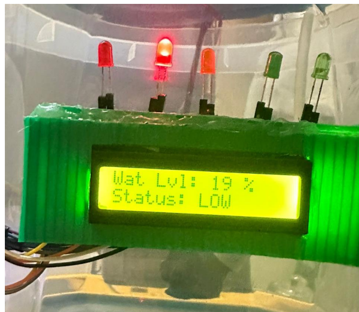
Figure 71: One of the red LED lights switched on and LCD Display the output.
