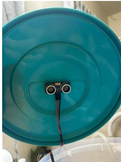
Figure 7: Ultrasonic sensor HC-SR04 placed under the water tank model cap.
