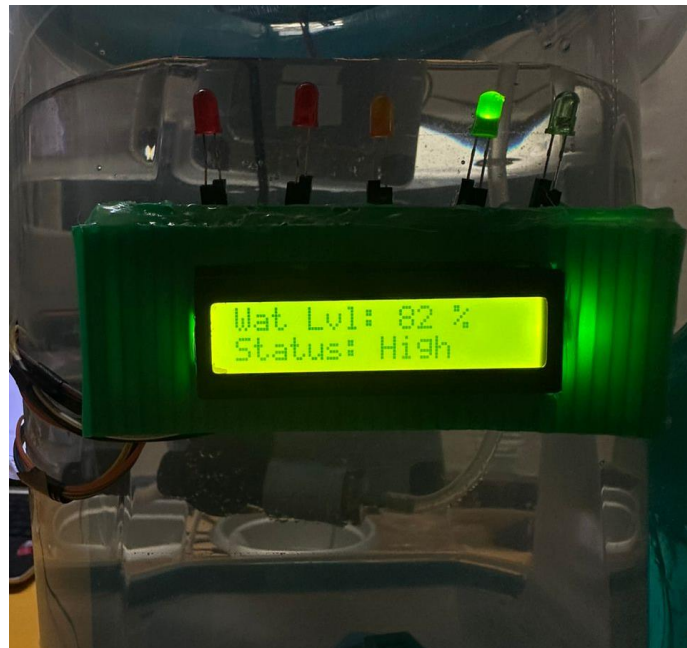
Figure 57: LCD display the output of the water level percentage and status.
