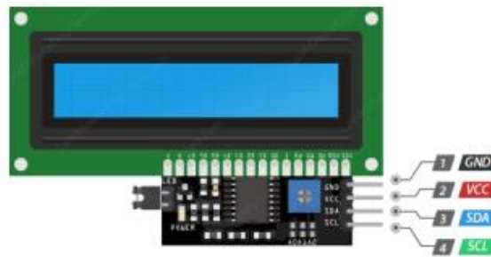
Figure 14:12C LCD Display pinouts.
