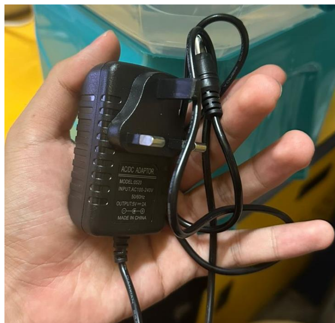
Figure 18: 5V DC Power Supply
