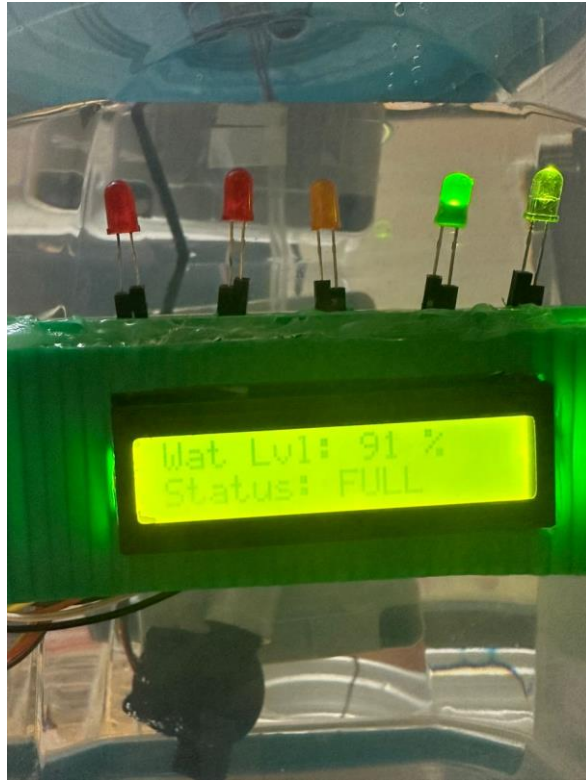
Figure 52: LCD display output for Full Level
