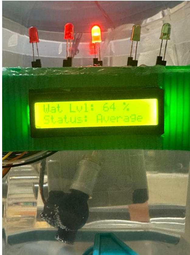
Figure 65: Orange LED switched on and LCD Display the output of the water level percentage and water status.
