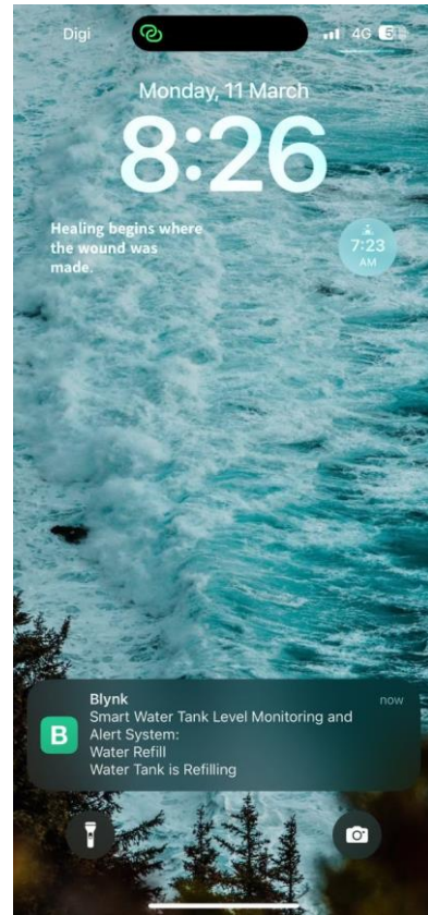
Figure 62: Notification of water refilling (water flow presence)
