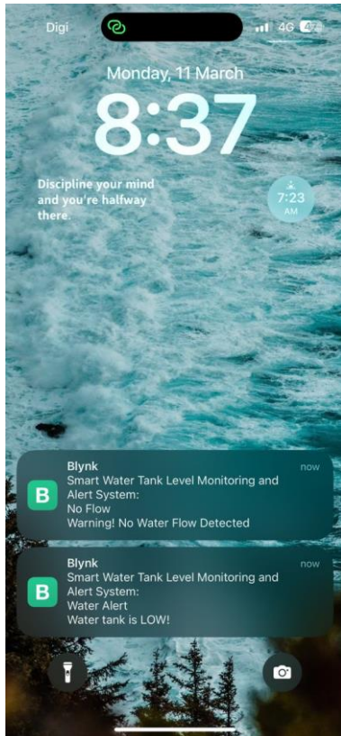
Figure 66: Notification for Low water level
