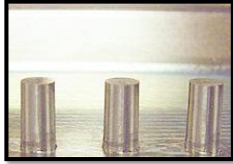
Figure 3.8: Pin Specimens (diameter 6mm, length 10mm)
