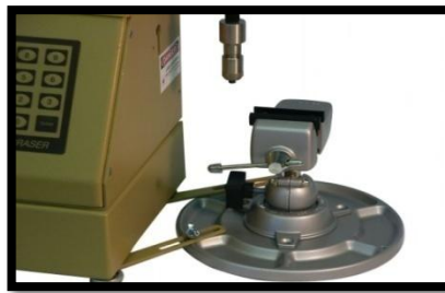
Figure 3.1: Universal Specimen Table of TABER® Linear Abraser
