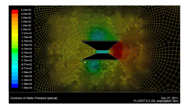
Figure 15: Pressure Contour
