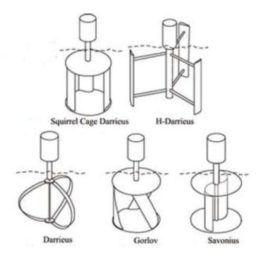
Figure 2: Vertical axis turbines [3]
