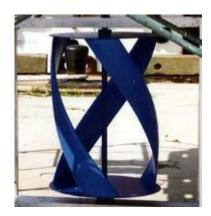
Figure 6: Gorlov Helical Turbine
