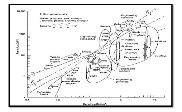
Figure 3: Ashby material selection chart: strength vs. density [8]
