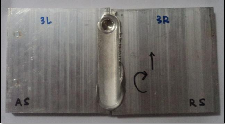
Figure 26: Sample 3, FSW plates (Round tool, 100 mm/min)
