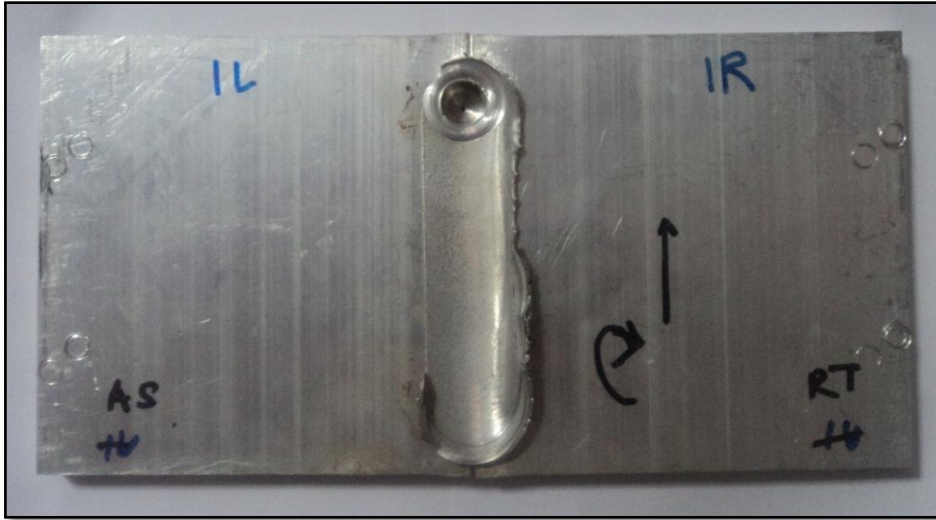
Figure 24: Sample 1, FSW plates (Round tool, 50 mm/min)
