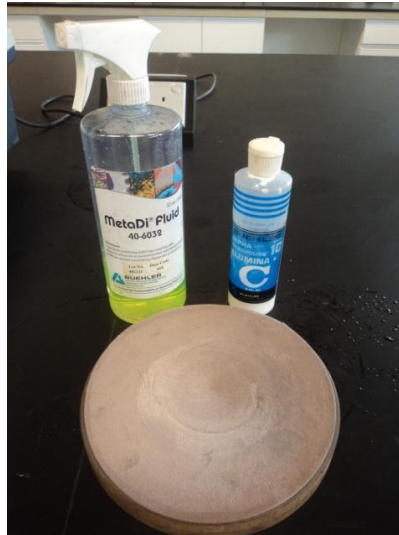
Figure 19: Tri-cloth, Metadi fluid & diamond paste
