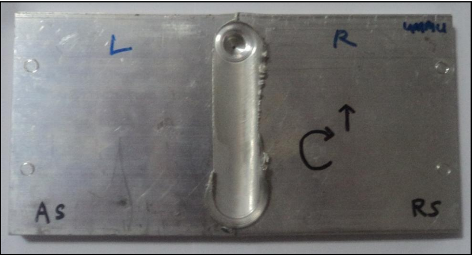
Figure 27: Sample 4, plates (Triangular tool, 50 mm/min)
