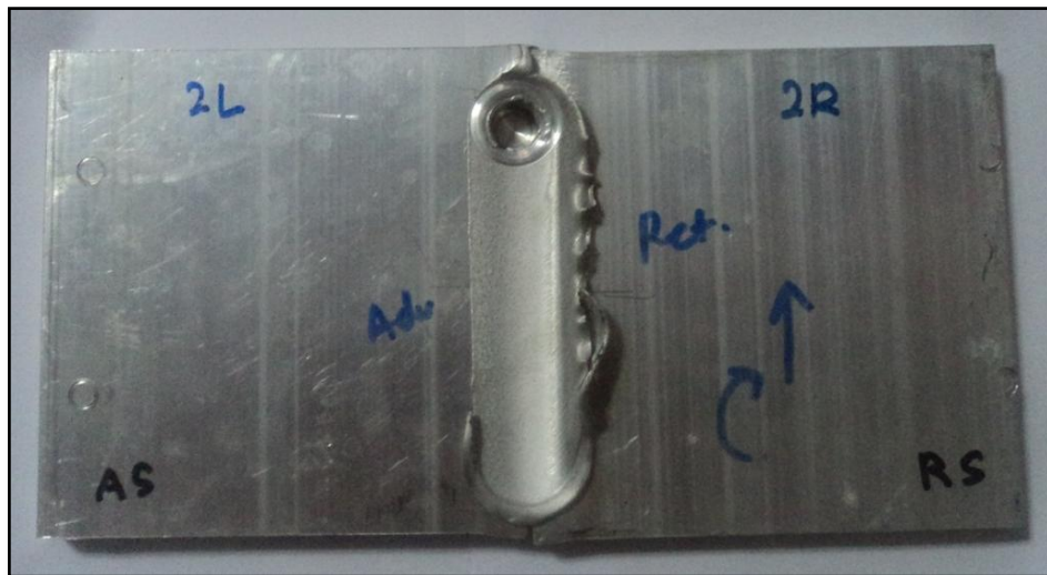
Figure 25: Sample 2, FSW plates (Round tool, 75 mm/min)
