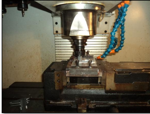
Figure 15: Workpiece undergo FSW process
