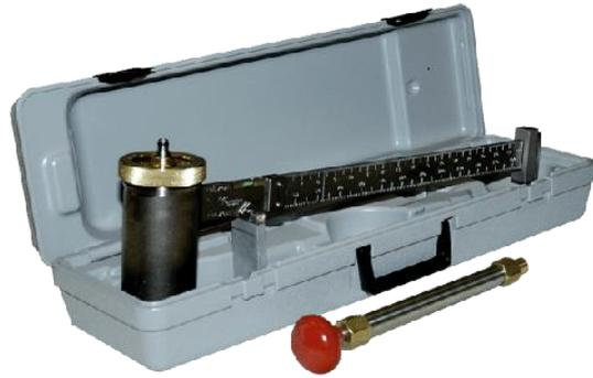
**FIGURE 9: PRESSURIZED MUD BALANCE**
