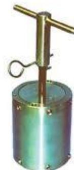
**FIGURE 7: HPHT FILTER PRESS TESTER**
