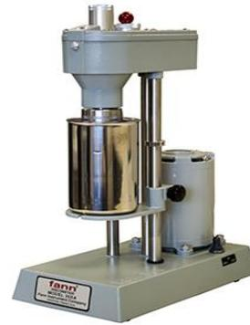
**FIGURE 8: MODEL 35 FANN VISCOMETER**
