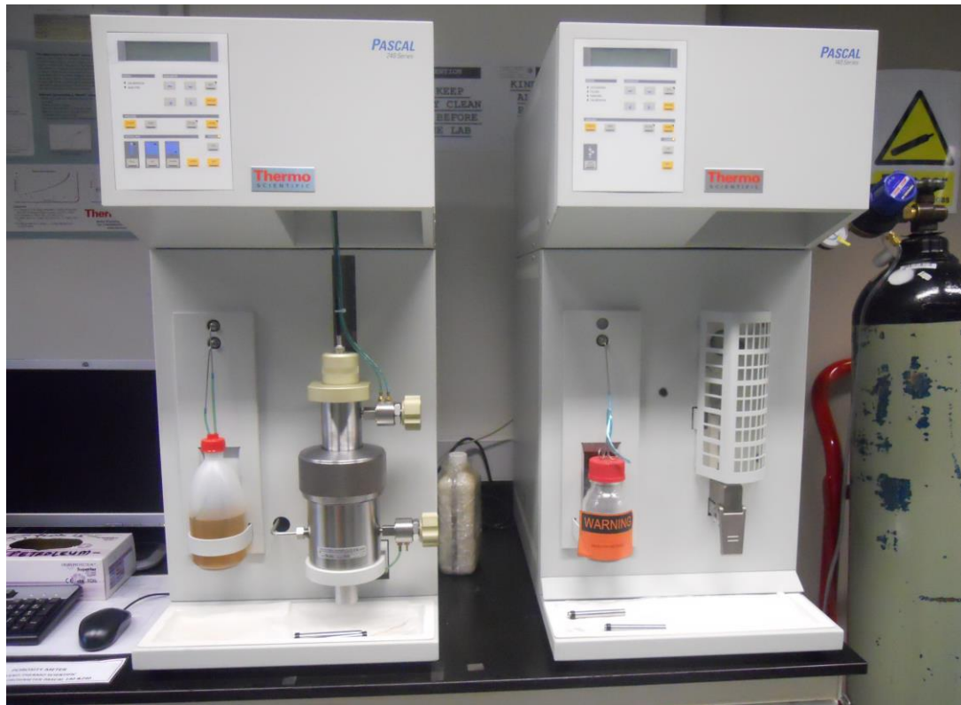
Figure 20: Poro-perm equipment provided in UTP laboratory
