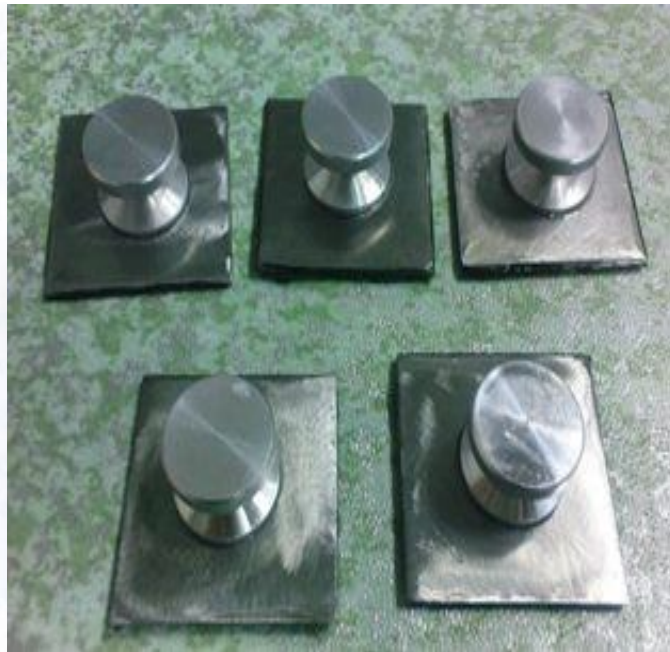
Fig. 3.9b Dolly attached to samples
