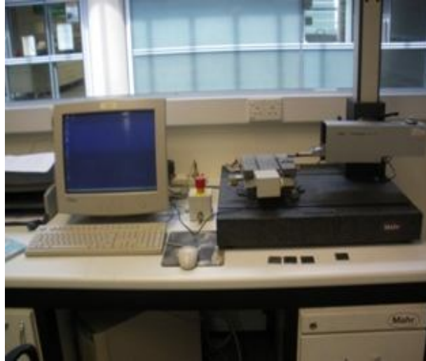
Fig.3.2 Profilometer used : Mahr. Perthometer
