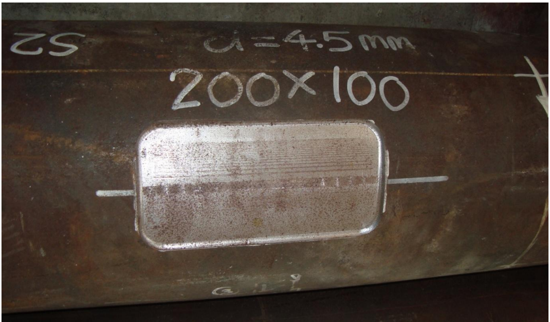
Plate D.2 Simulated defect
