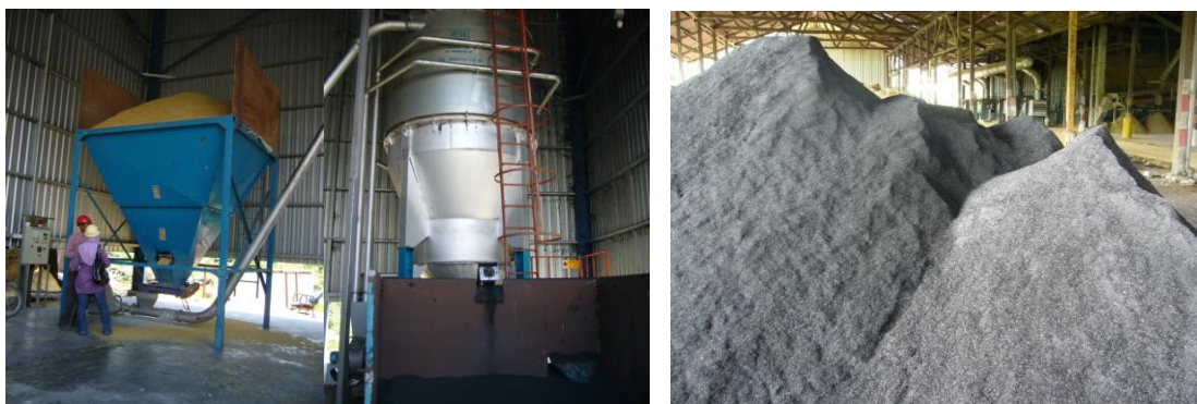
Figure 3.1 Cyclonic Husk Furnace (CHF) & SGM-RHA
