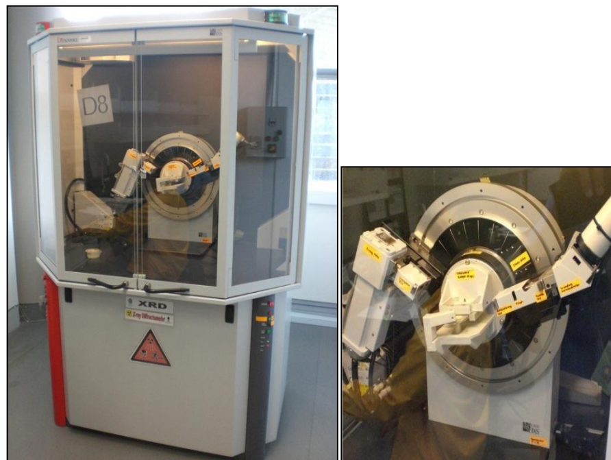
Figure 3.11 Bruker Axs D8 Advance X-Ray Diffractometer
