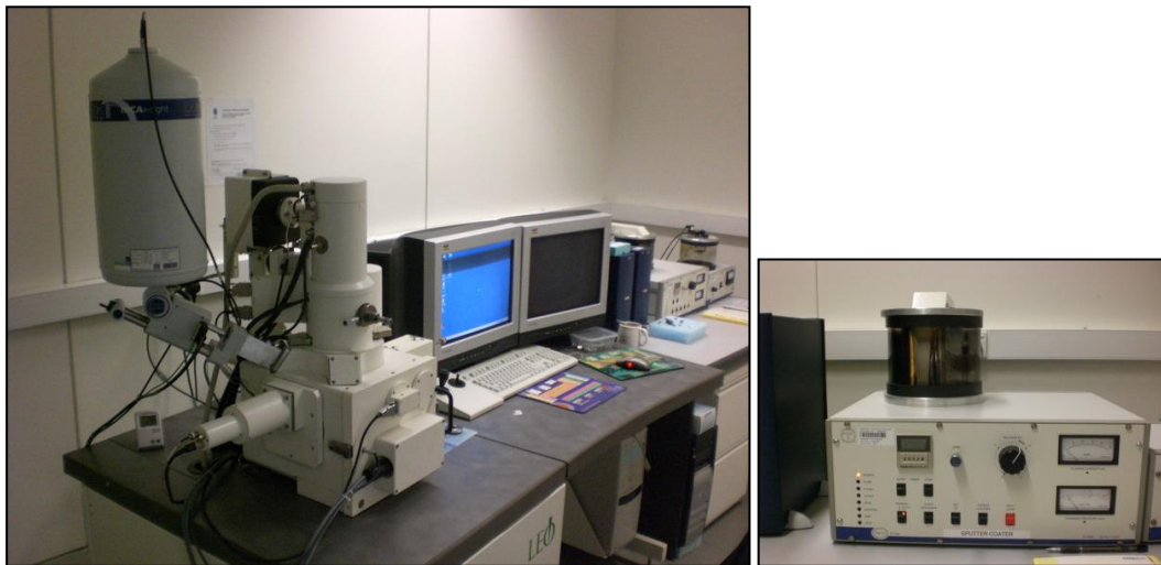
Figure 3.15 LEO 1430 VP Inca X-Sight Oxford SEM Instrument with Sputter Coater.
