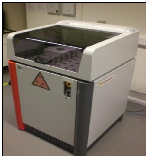
Figure 3.10 Bruker Axs S4 Pioneer X-Ray Spectrometer
