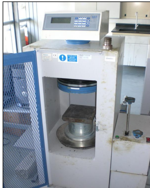
Figure 3.12 Digital Compressive Testing Machine
