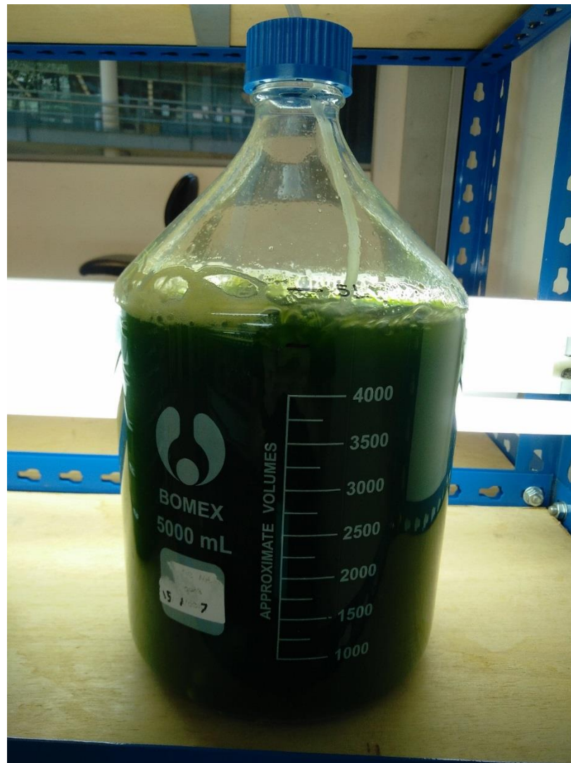
Figure 3.2: Chlorella vulgaris culture in the 5-L functional bioreactor.
