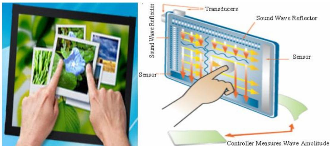
Figure 2.2: SAW display device (left) and the architecture of SAW display (right)
