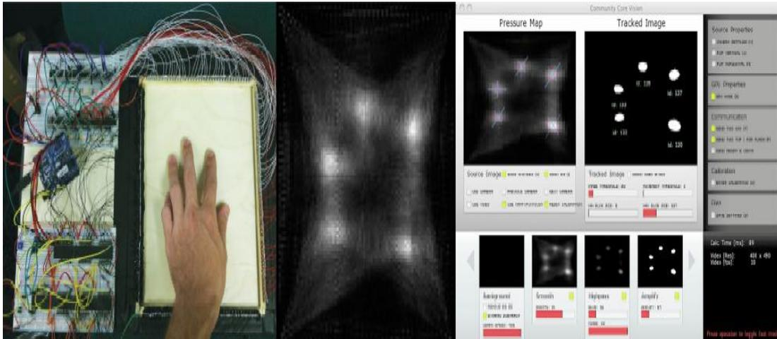
Figure 2.12: Architecture of the Scanning FTIR display (left) and fingertip calibration (right) (Moeller & Kerne, 2010)
