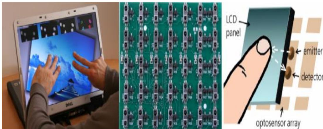
Figure 2.10: ThinSight display (left) and its architecture (left) (Izadi, et al., 2007)
