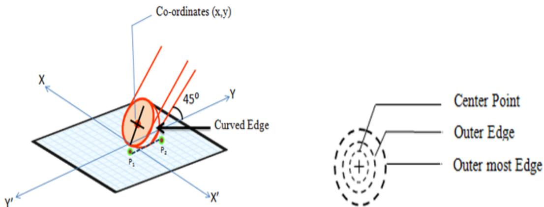
Figure 5.2: Geometric model of a fingertip using the oblique touch
