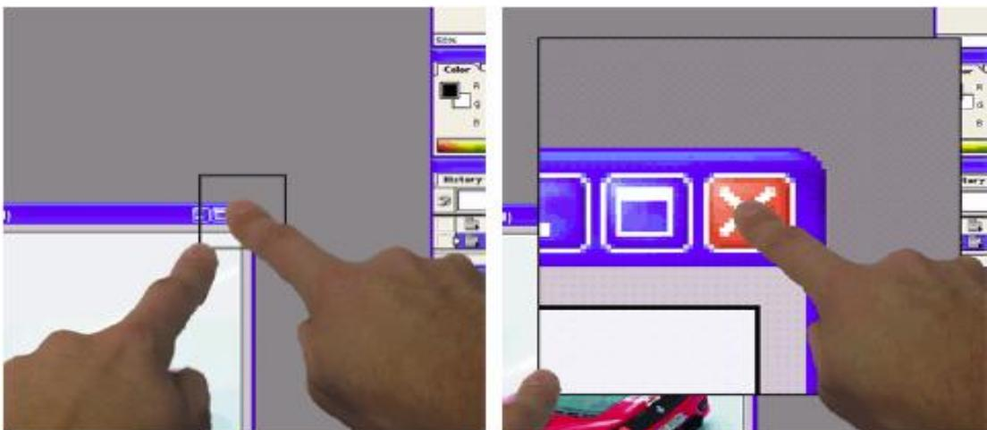
Figure 2.15: Dual finger stretch technique (Hrvoje Benko, et al., 2006)
