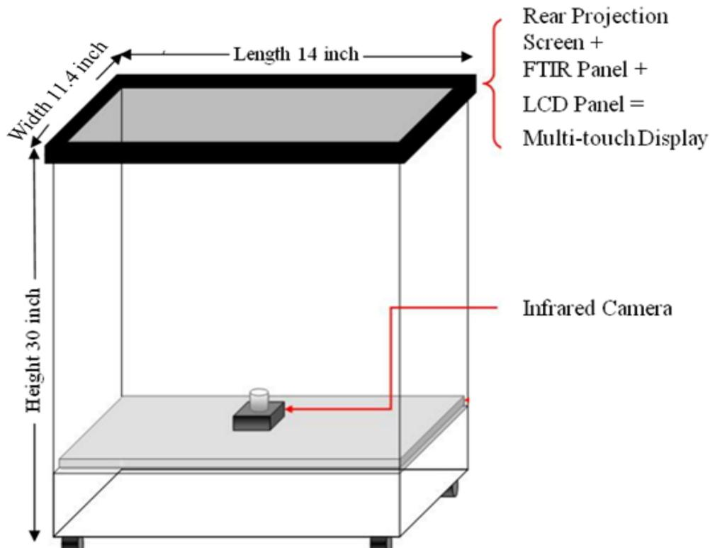
Figure 4.7: LCD panel based multi-touch tabletop display
