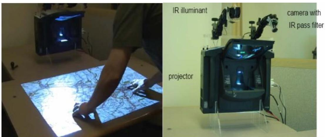
Figure 2.5: PlayAnywhere display (left) and its architecture (right)(Wilson, 2005)
