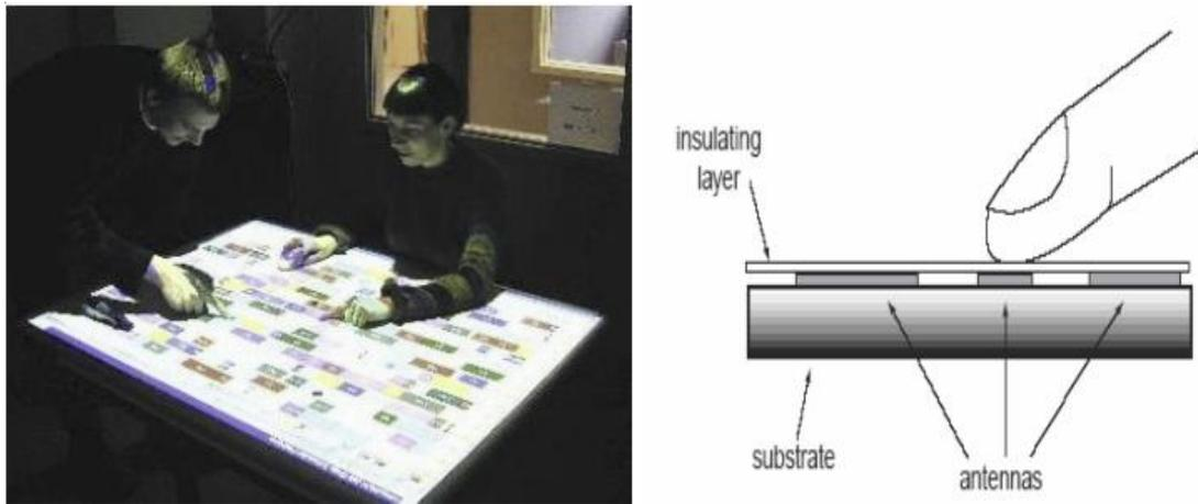
Figure 2.3: DiamondTouch display (left) and its architecture (right) (Dietz & Leigh, 2001)
