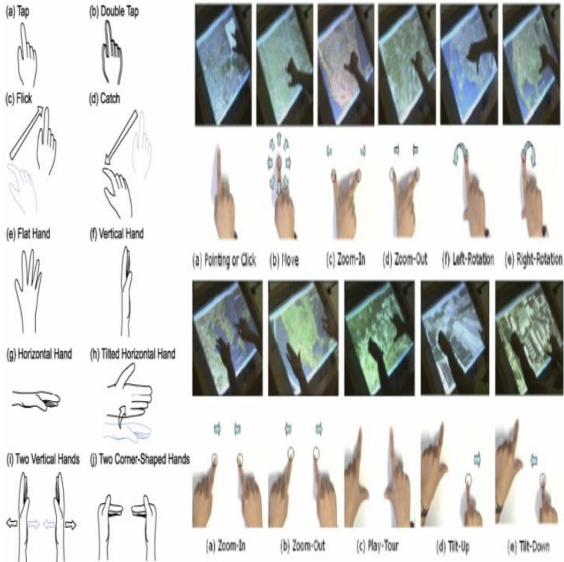
Figure 2.23: One and two handed multi-touch interaction with interactive displays
