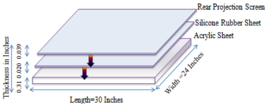
Figure 4.14: Overlaid layers on the acrylic sheet
