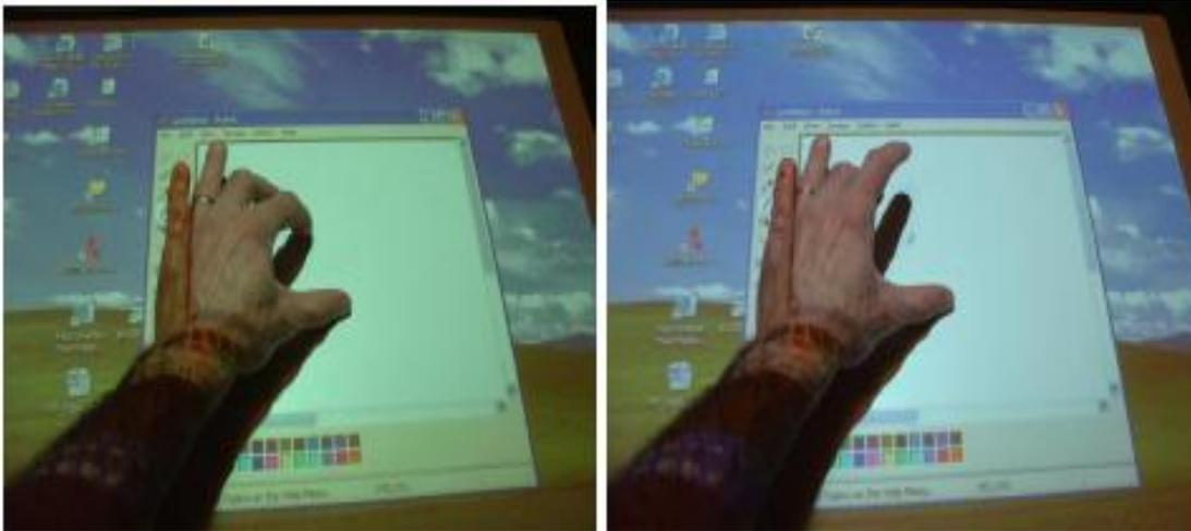
Figure 2.13: The fluid DTMouse technique (Esenther & Ryall, 2006)
