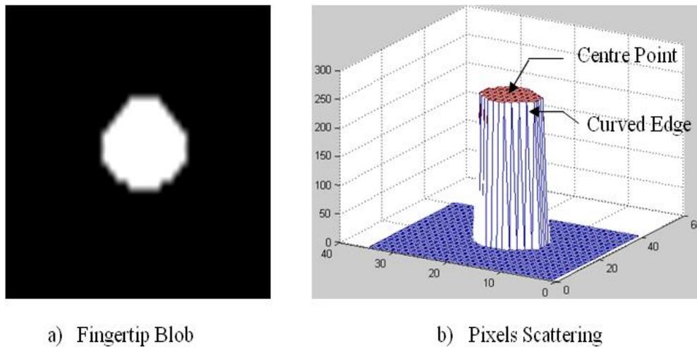
Figure 5.4: Fingertip Blob (a) and its Pixel Scattering (b) for vertical touch
