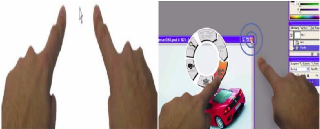
Figure 2.14: Dual finger midpoint and X-Menu technique (Hrvoje Benko, et al., 2006)
