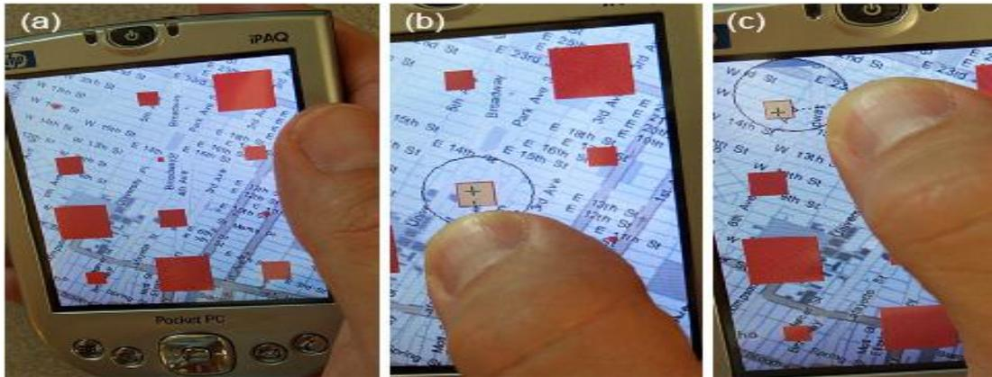
Figure 2.17: The Shift technique with callout function that is activated only when a user aims to select small target elements (Vogel & Baudisch, 2007)
