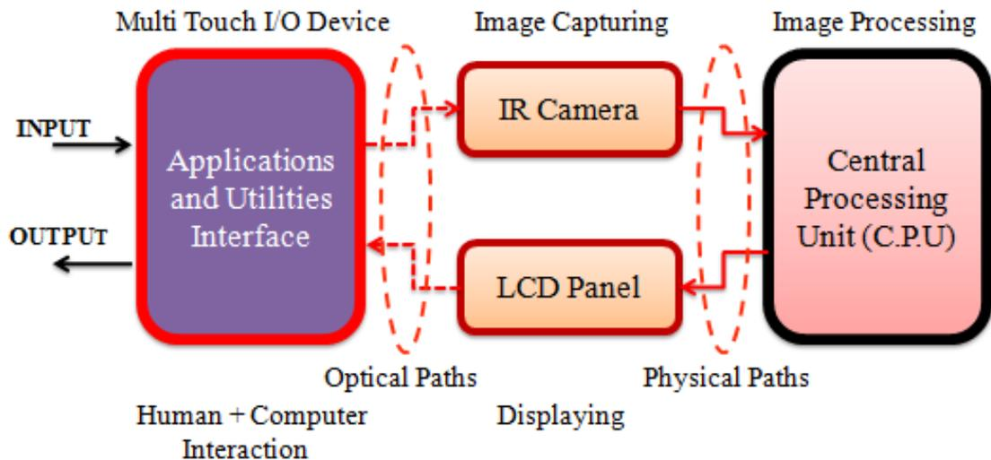
Figure 4.2: Layout of the multi-touch tabletop display architecture
