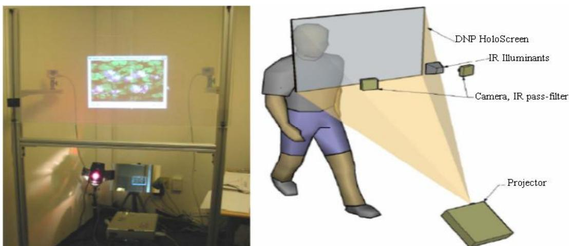
Figure 2.6: TouchLight display (left) and its architecture (right) (Wilson, 2004)
