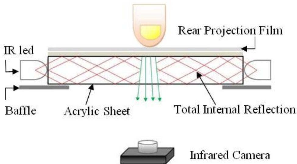
Figure 4.5: FTIR panel with configuration of IR LEDs
