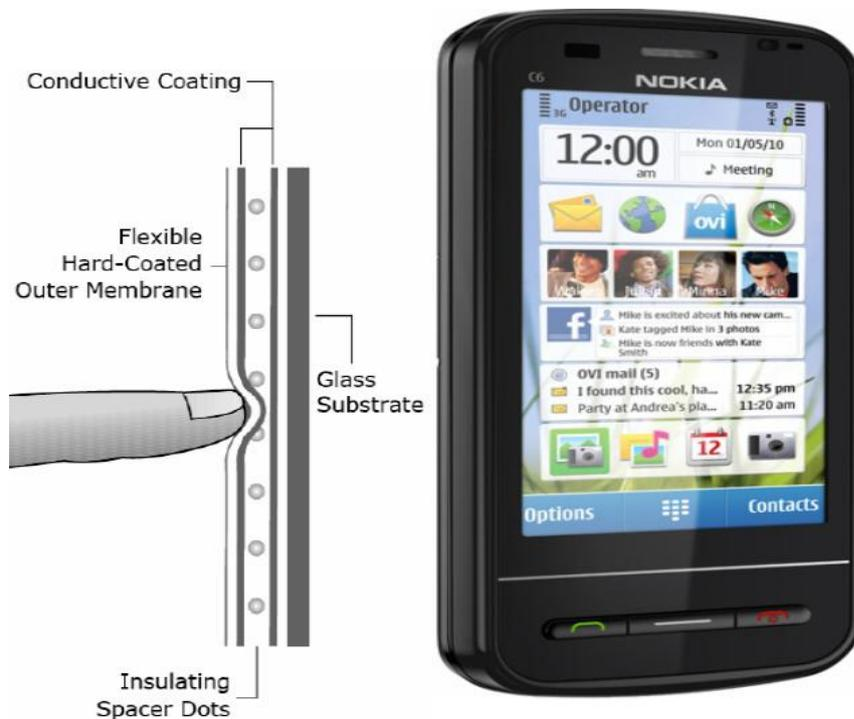
Figure 2.1: Architecture of resistive display (left) (Schöning, et al., 2008) and resistive display device (right) (Lutherz, 2011)
