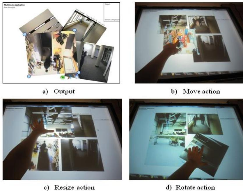
Figure 4.20: Direct gesture of fingers on the multi-touch tabletop display
