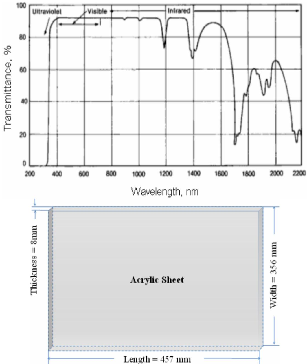
Figure 4.3: Transmission capability of acrylic sheet (top) (ASM, 2003) and its specifications (bottom)
