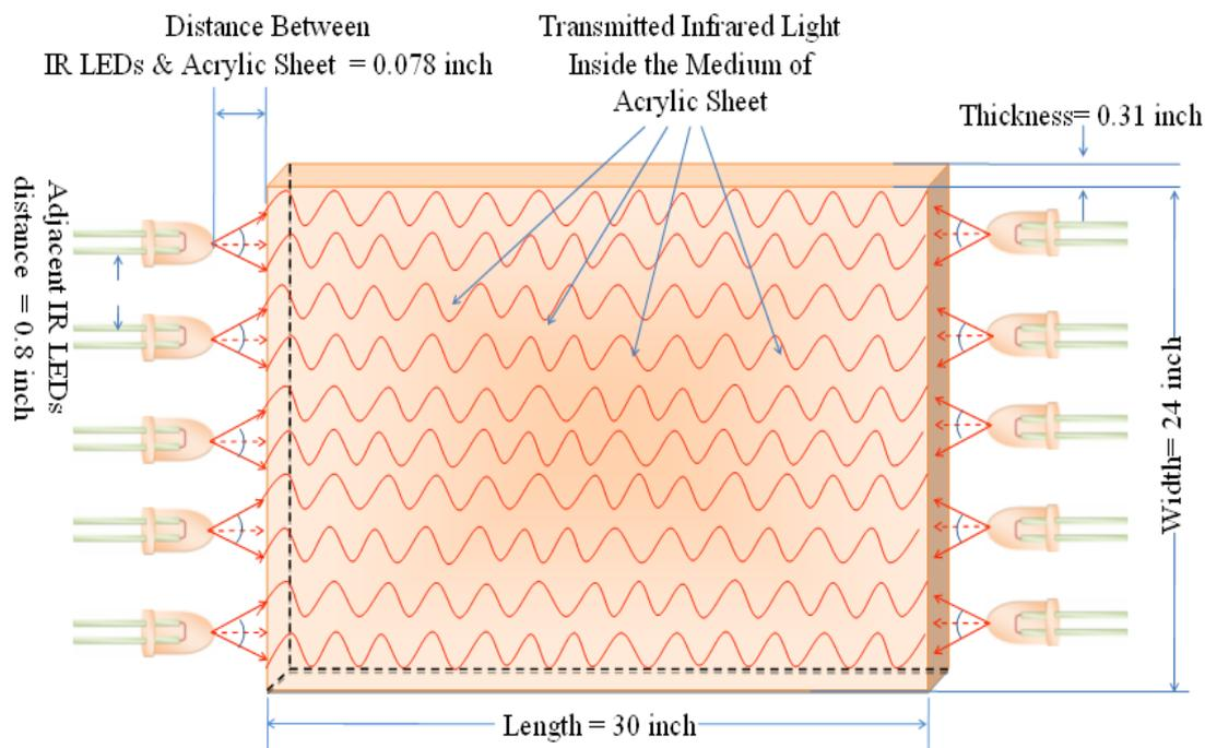
Figure 4.15: Layout of the internal architecture of the optical panel
