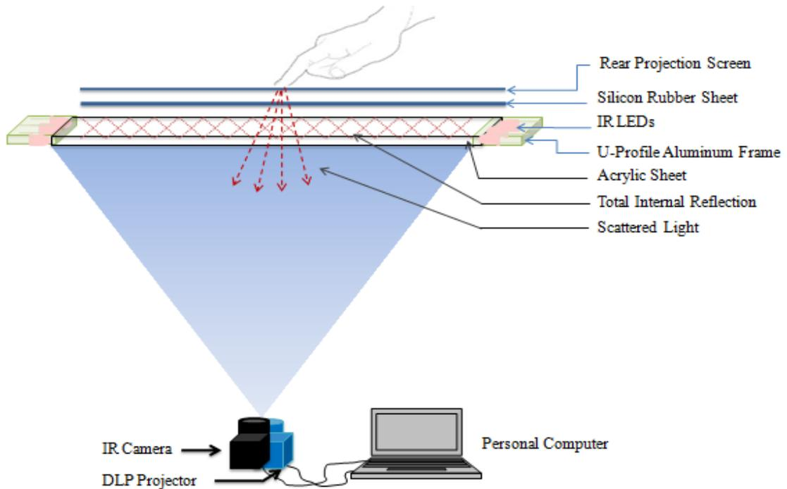
Figure 4.16: Layout of the internal architecture of the multi-touch tabletop display
