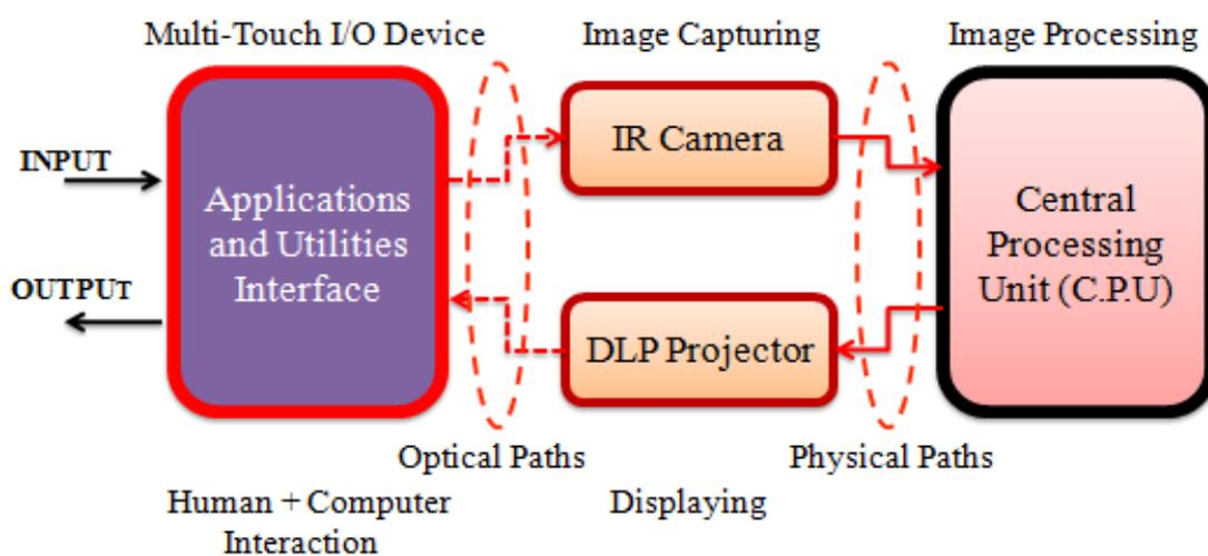
Figure 4.13: Layout of the architecture of the multi-touch display
