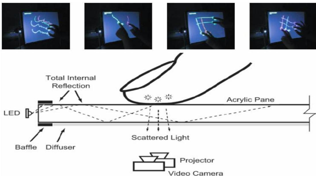
Figure 2.7: Multi-touch display (above) and its architecture (below) (J. Y. Han, 2005)
