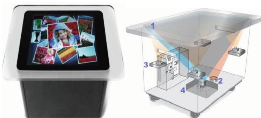
Figure 2.9: MS surface (left) and its architecture (right) (Microsoft Inc, 2007)
