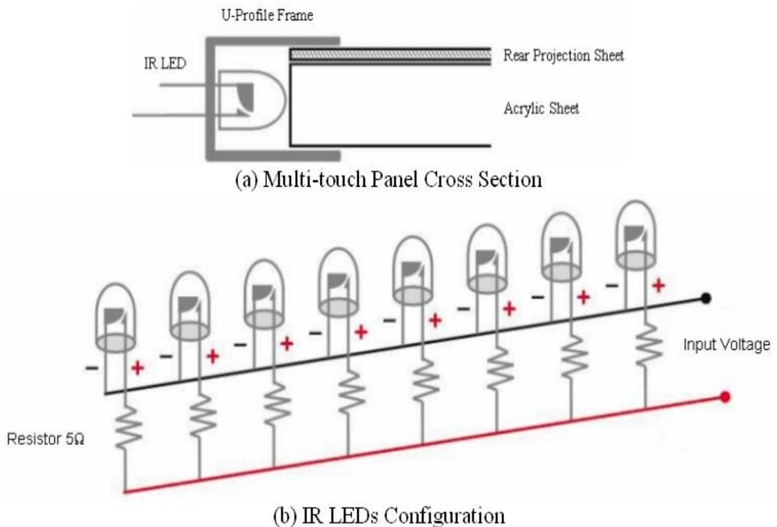
Figure 4.4: Multi-touch panel cross section and IR LED configuration
