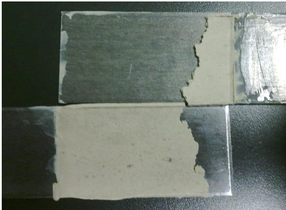
Figure 4. 32: The interfacial failure of F4
