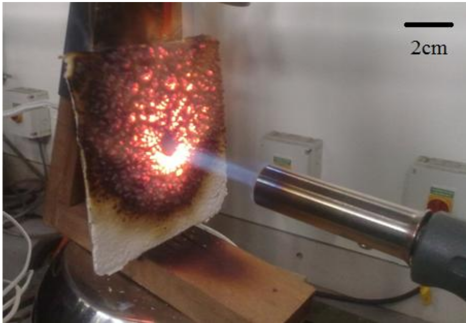
Figure 4. 23: After fire started, F1 starts to swell.
