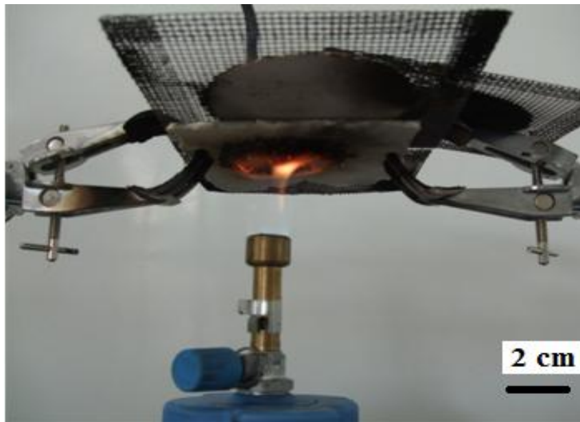
Figure 3. 2: Coating was faced downwards with vertical Bunsen burner
