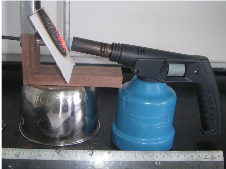
Figure 3. 3: Second trial of fire protection test.
