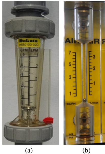
Figure 4.2: Rotameters (a) Polysulfone-Water and (b) Acrylic-Air.
