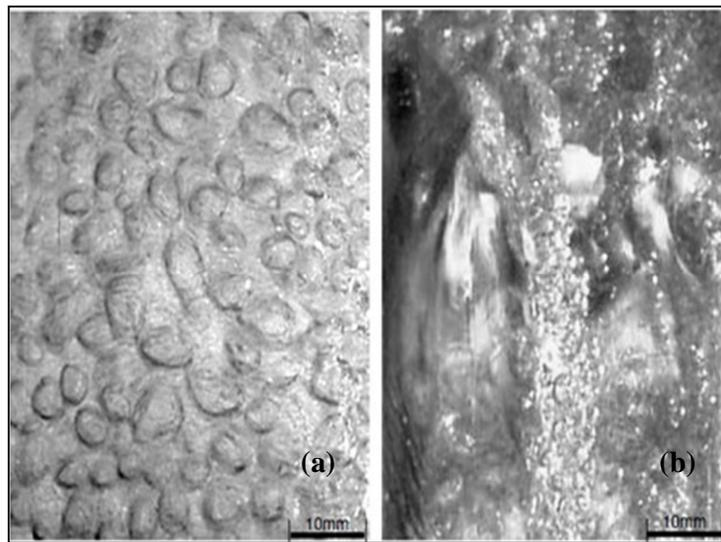
**Figure 2.10:** Photographs of (a) Homogeneous and (b) Churn-Turbulent Flow [51].
