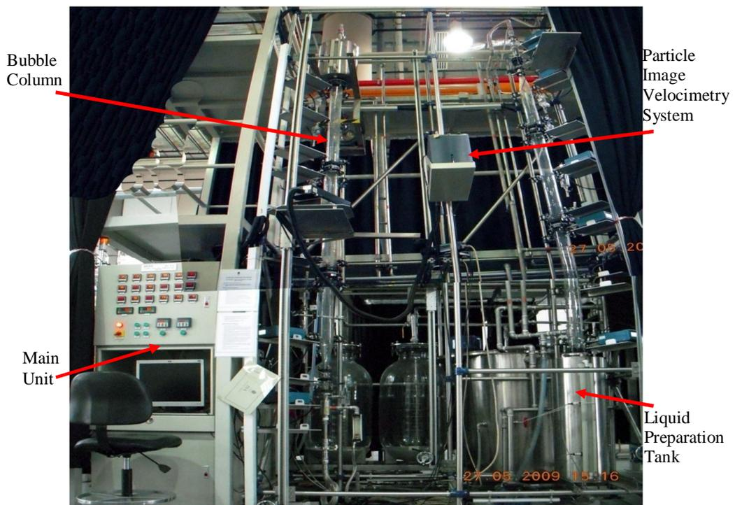
**Figure 2.3:** Co-Current Bubble Column Pilot Plant.
