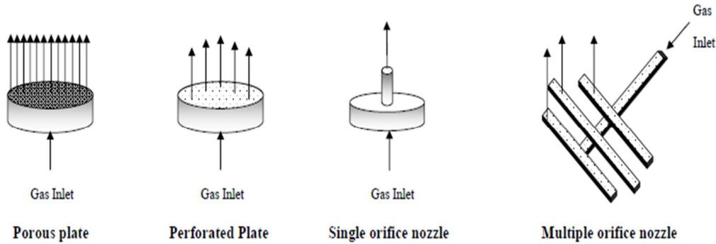
**Figure 2.5:** Different Types of Gas Distributors Employed in Bubble Column [19].
