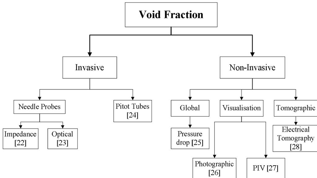
**Figure 2.6:** Different Invasive and Non-invasive Techniques to Measure Void Fraction.
