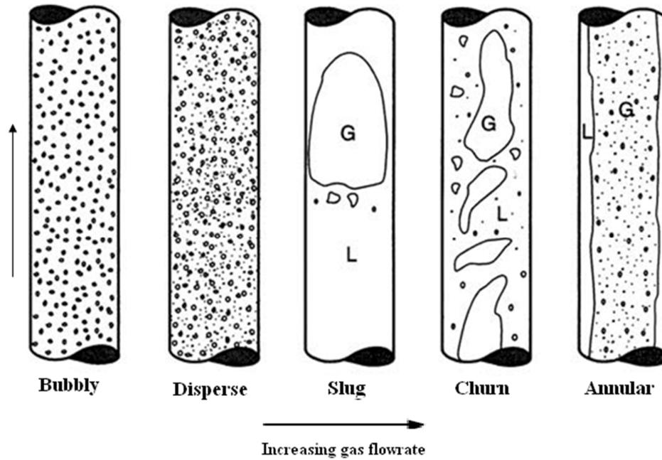
**Figure 2.8:** Flow Regimes in Vertical Co-Current Bubble Column [42].
