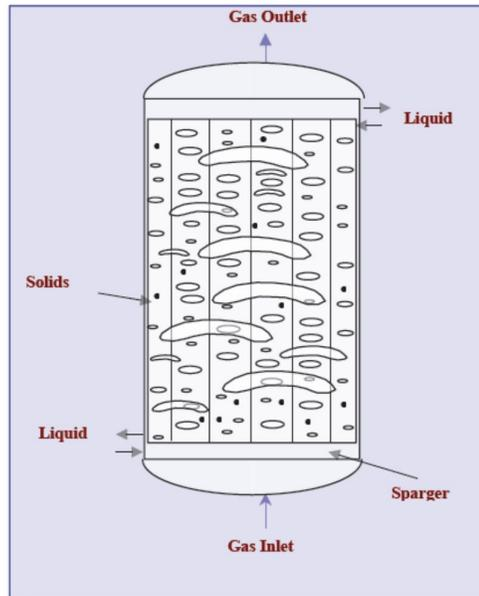
**Figure 2.1:** Schematic Diagram of Bubble Column [8].
