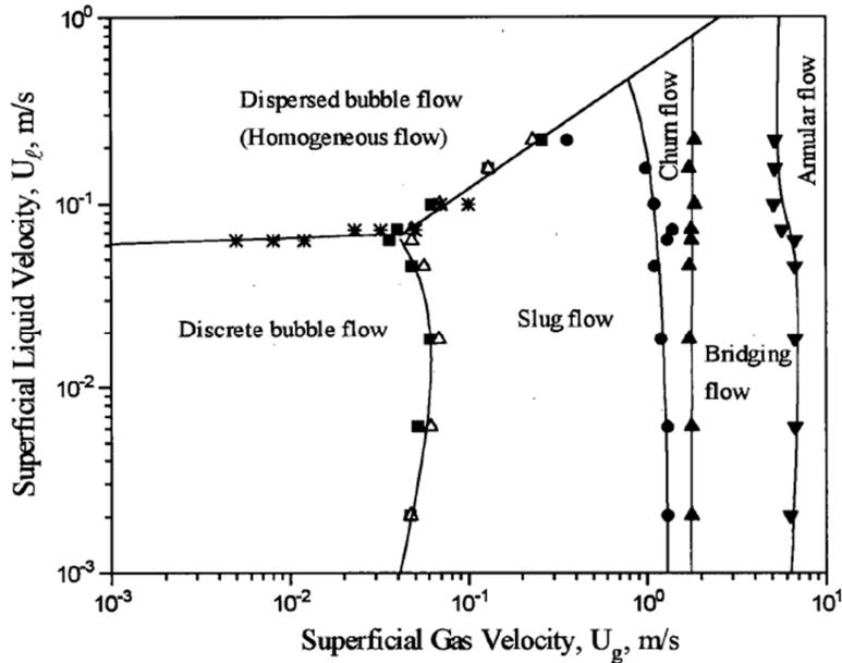
**Figure 2.9:** Bubble Column Flow Regime Map for Air-Water System [45].
