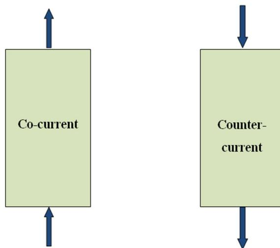
**Figure 2.2:** Direction of Flow in a Bubble Column.
