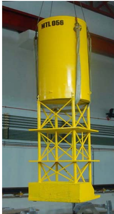
Figure 5.3: Truss spar model (Phase 1)
