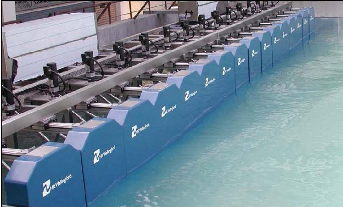
Figure 5.8: UTP basin wave maker system (Source: UTP basin user manual, HR Wallingford, 2008)
