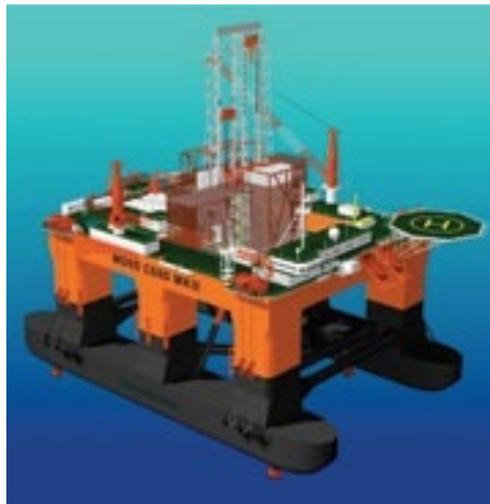
Figure 2. 6 The sixth generation semi-submersible platform [17]
