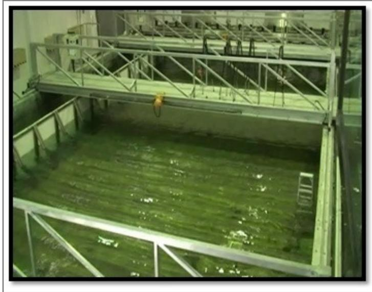
Figure 3. 9 Wave tank filled with water
