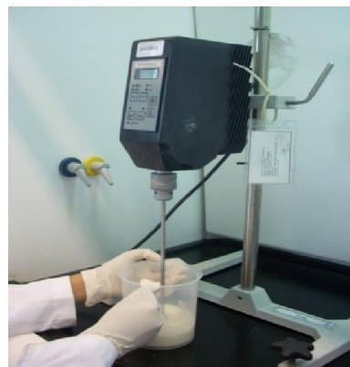
Figure 3.10: Mixing process of intumescent coating using Shear Mixer
