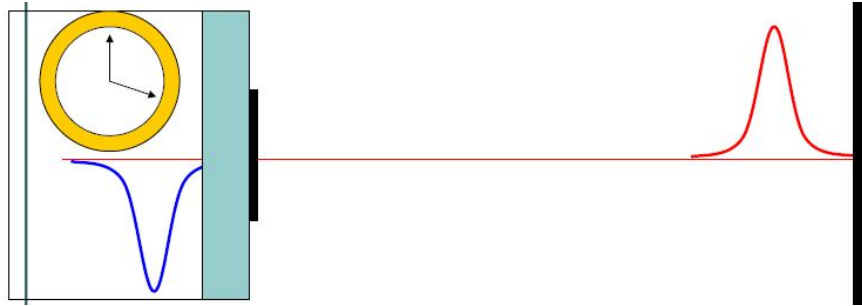
Figure 2.9 Timed Pulse EDM (Range = Time x Speed of light / 2 = \frac{1}{2} c \cdot \Delta t ) (Source: M. Ted and W. Brain, 2007)
