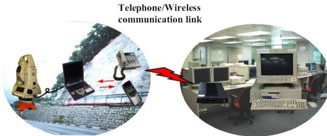
Figure 2.7 Real Time Monitoring System. (Source: A. Chrzanowski, G. Bastin and R. Wilkins, 2003)
