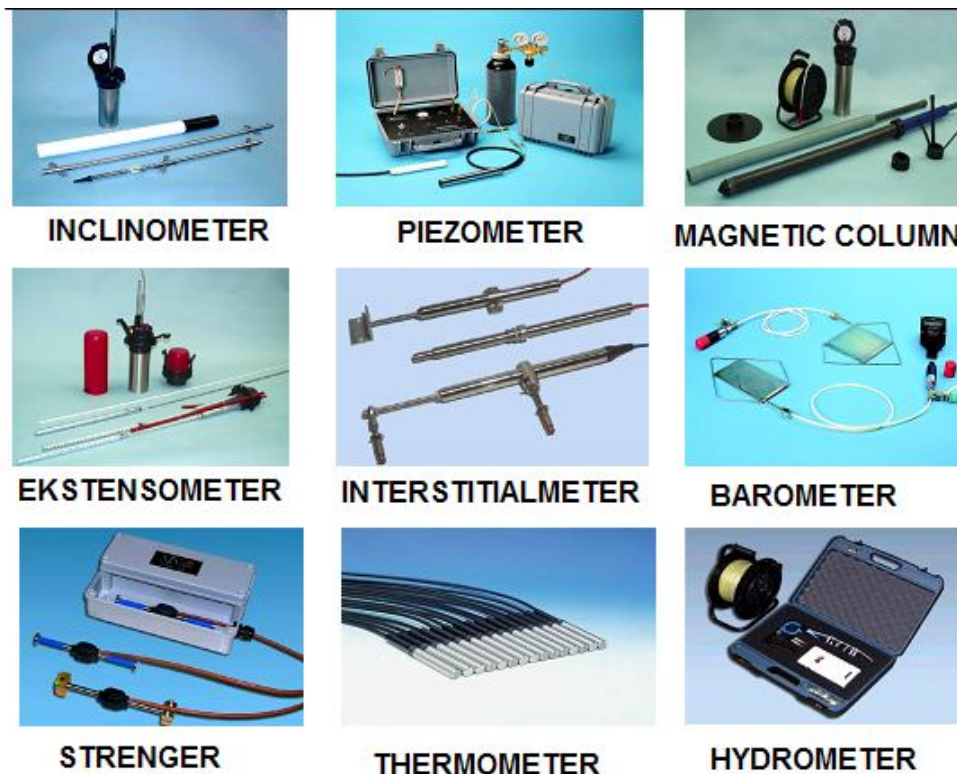
Figure 2.6 Geotechnical Methods and Special Instruments (Source: C.D. Hill, and K.D Sippel M, 2002)
