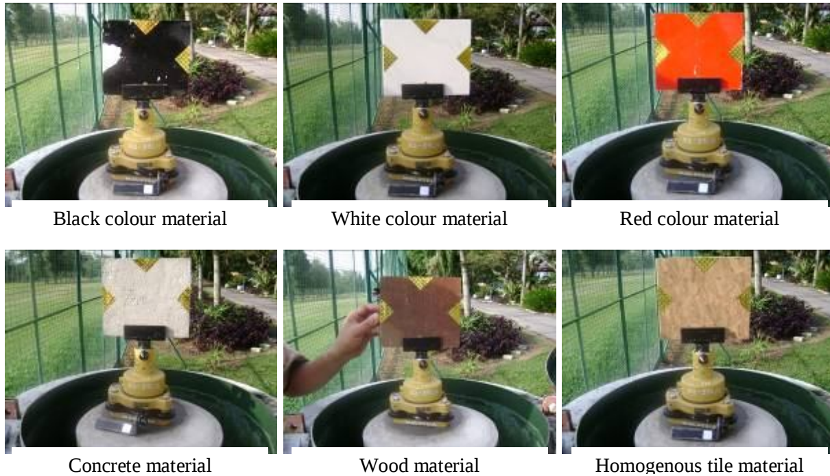
Figure 3.3 Various target reflectors used in this research
