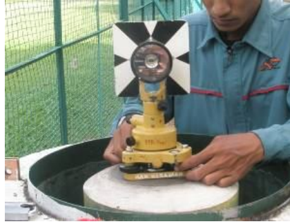
Figure 3.4 A standard single prism used in this research
