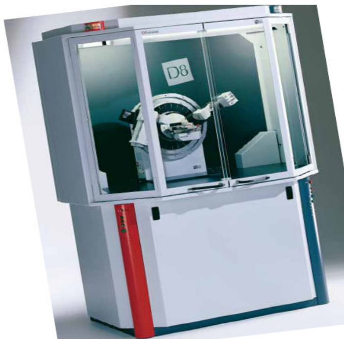
Figure-58: Photograph of the XRD BRUKER apparatus (Model number =D8 ADVANCE) used in the experiment
