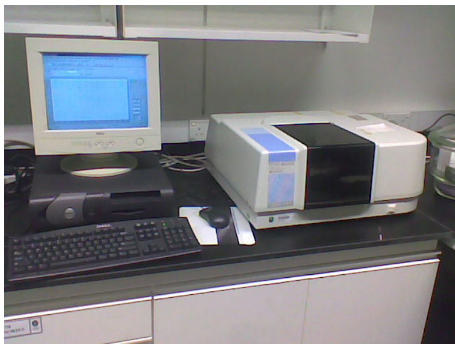
Figure-59: Photograph of the FT-IR from Perkin-Elmer (Model number = Spectrum one) used in the experiment.
