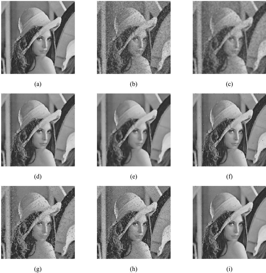
Figure 5.13 Noisy 256x256 8-bit grayscale Lena image corrupted by 0.2 uniform impulse noise filtered by: (a) the proposed filter, (b) 3x3 average filter, (c) 5x5 average filter, (d) 3x3 median filter, (e) 5x5 median filter, (f) EIE, (g) WFM, (h) GFIF, and (i) FRINR.
