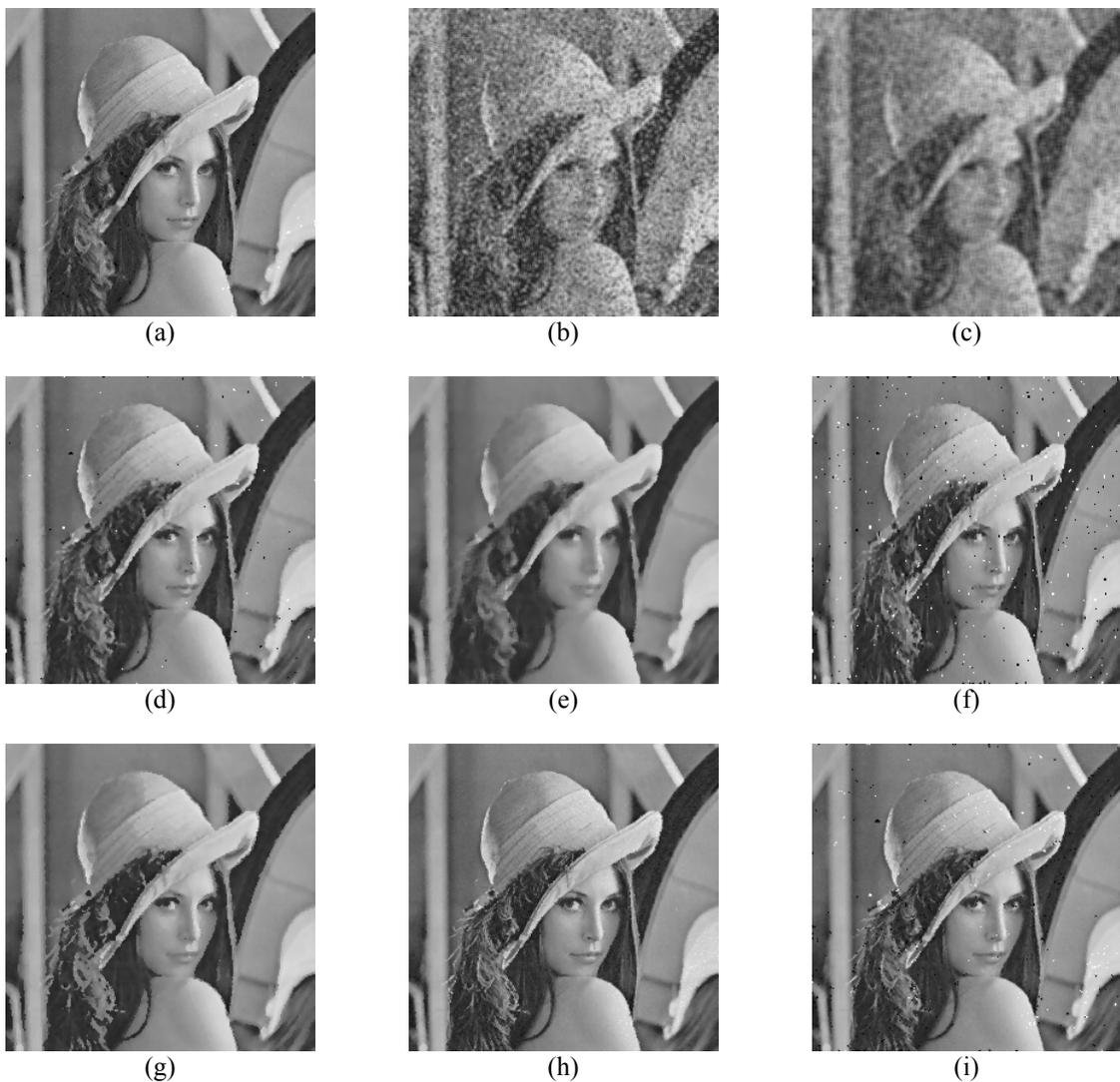
Figure 5.10 Noisy 256x256 8-bit grayscale Lena image corrupted by 0.2 salt-and-pepper noise filtered by: (a) the proposed filter, (b) 3x3 average filter, (c) 5x5 average filter, (d) 3x3 median filter, (e) 5x5 median filter, (f) EIE, (g) WFM, (h) GFIF, and (i) FRINR.
