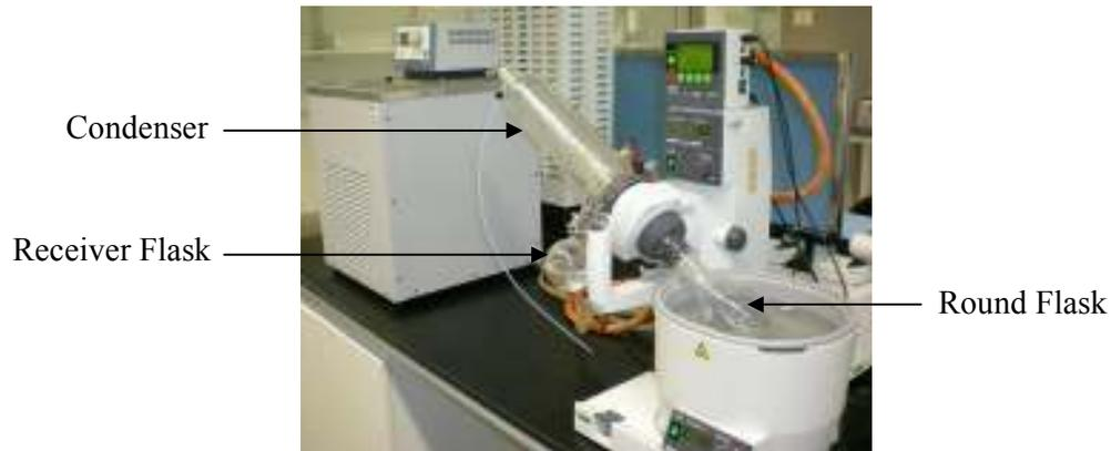
**Figure 3.6** Separation of hexane from biodiesel using rotary evaporator
