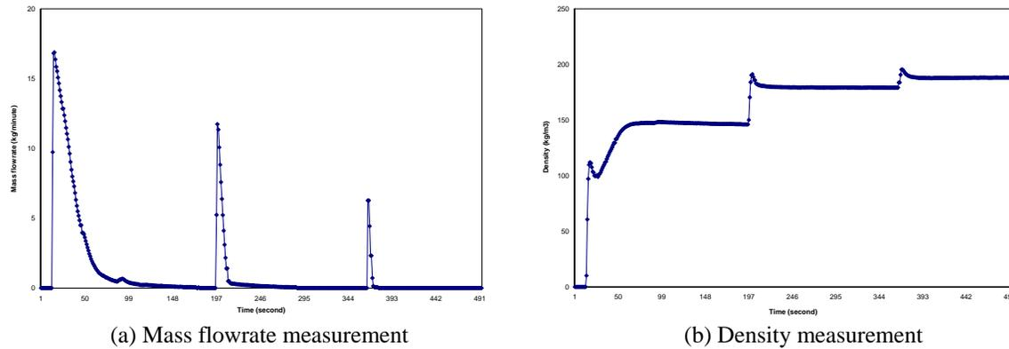
Figure 2.31: Coriolis measurements using Micro Motion flowmeter
