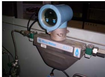
Figure 2.25: Micro Motion coriolis flowmeter
