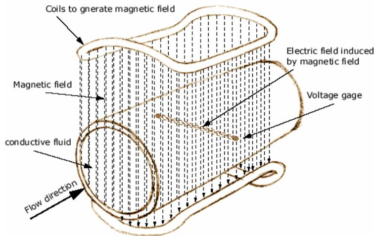
Figure 2.17: Inline magnetic flowmeter [38]
