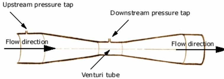
Figure 2.4: Venturi tube flowmeter [4]
