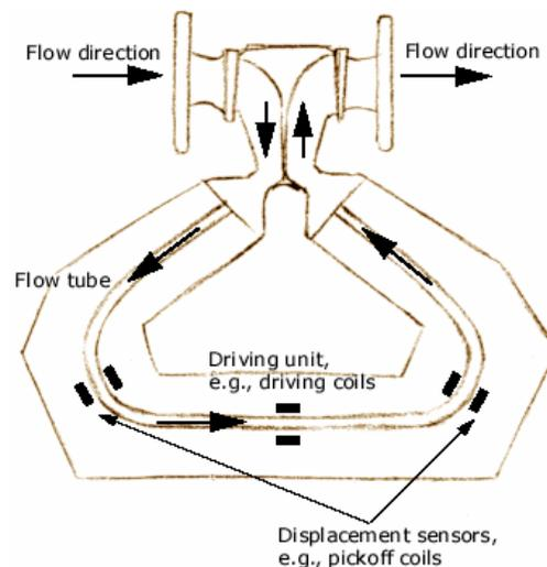
Figure 2.21: Coriolis mass flowmeter [237]
