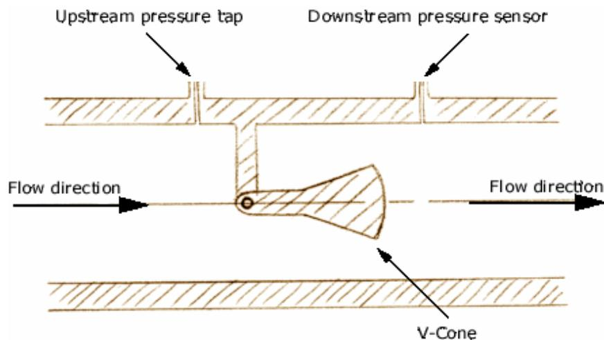
Figure 2.7: V-cone flowmeter [4]
