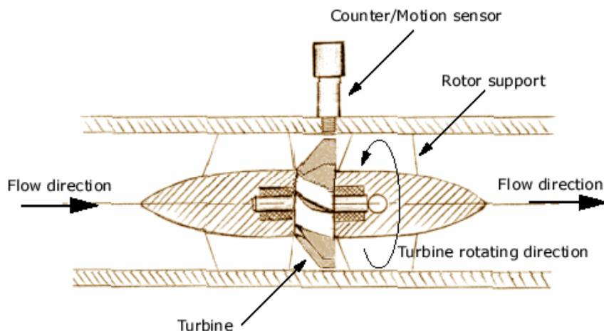
Figure 2.13: Turbine flowmeter [5]
