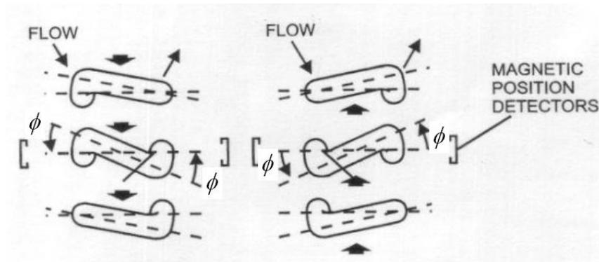
Figure 2.29: Deflection Angle Measurements [3]
