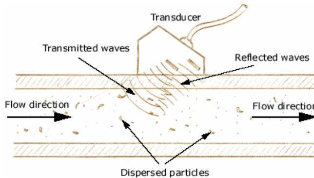
Figure 2.15: Doppler ultrasonic flowmeter [36]
