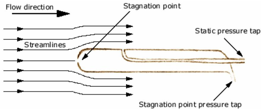
Figure 2.8: Pitot tube flowmeter [4]
