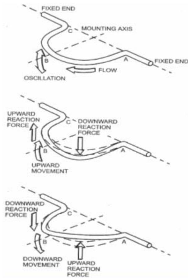
Figure 2.26: Coriolis principle [3]
