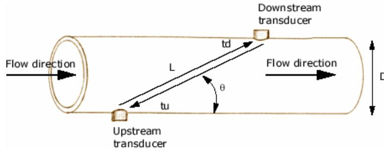
Figure 2.14: Transit time ultrasonic flowmeter [35]
