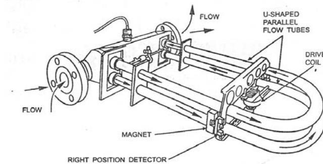
Figure 2.30: Typical construction of coriolis flowmeter [3]
