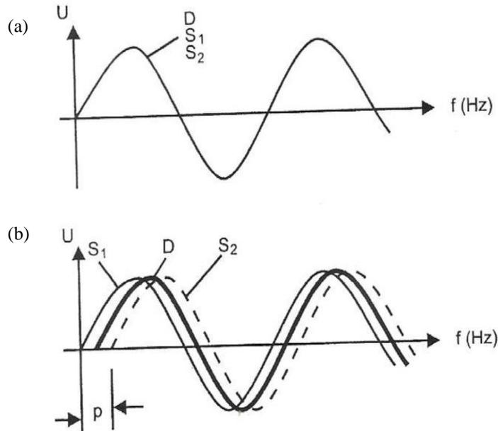
Figure 2.27: Sine waves (a) No Flow (b) Mass Flow [3]
