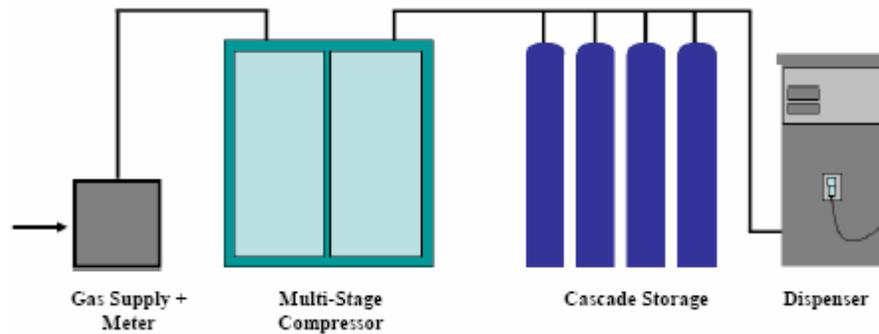
Figure 2.1: Fast-fill CNG filling station [2]
