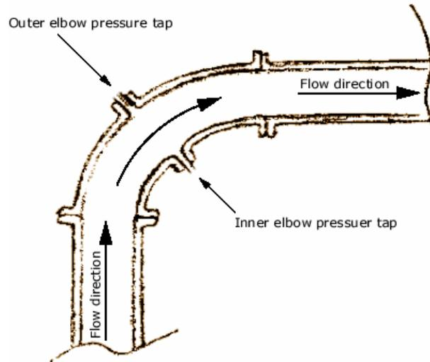
Figure 2.10: Elbow flowmeter [4]
