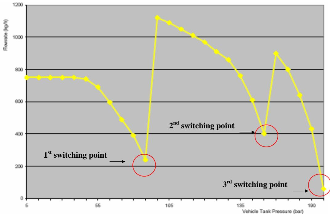
Figure 2.2: Mass flowrate during fast-filling for vehicle tank pressure (in bar) [2]
