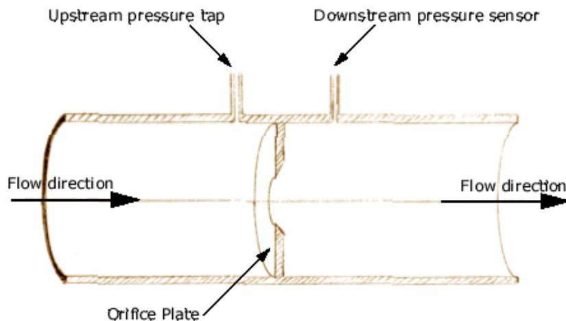
Figure 2.3: Orifice plate flowmeter [4]
