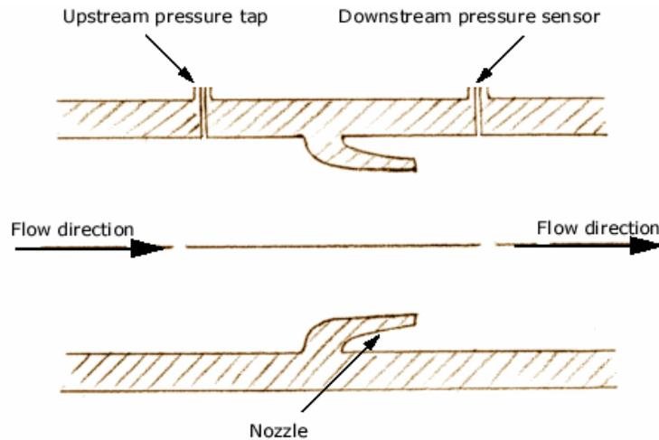
Nozzle shrinks down the cross-section area of the pipe and create pressure differential.
