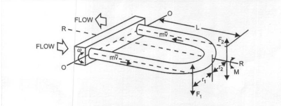
Figure 2.28: Oscillating U-tube [3]
