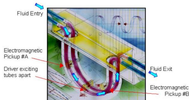
Figure 2.24: Coriolis in U-tube [42]
