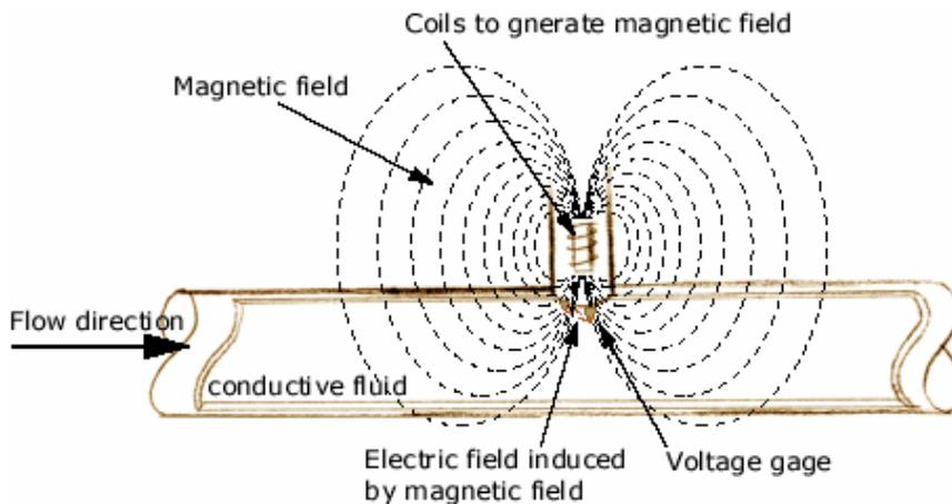
Figure 2.18: Insertion magnetic flowmeter [38]
