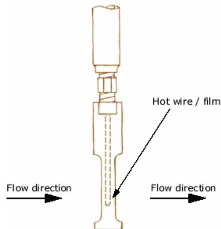
Figure 2.20: Thermal mass flowmeter [14]
