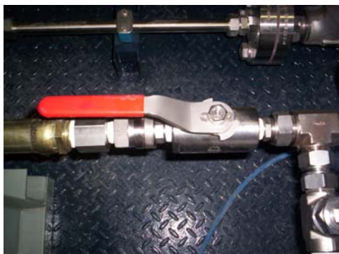
(c) The valve located at car cylinder bottom neck is turned to ‘ON’ position.
