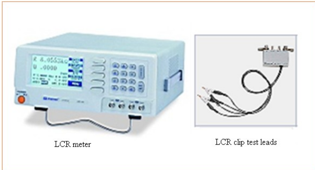
Figure 3.3: LCR meter for dielectric properties measurement
