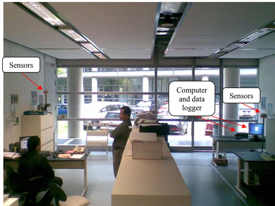
Figure 3.17 Lay out of the experiment location and sensors arrangement
