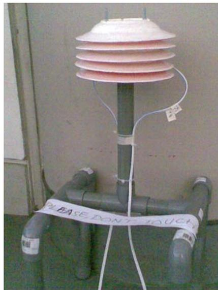
Figure 3.16 Construction of temperature and humidity sensors covered with 4 stage of white-painted plastic plate
