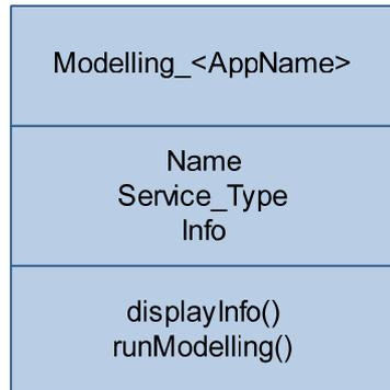
**Fig. 6.7** Modelling Service Provider class diagram
