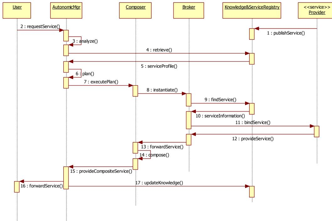
**Fig. 4.9** UML sequence diagram of the autonomous SOA
