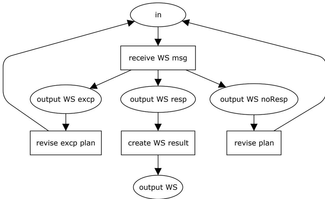
**Fig. 4.15** Petri Net model of the receive operation
