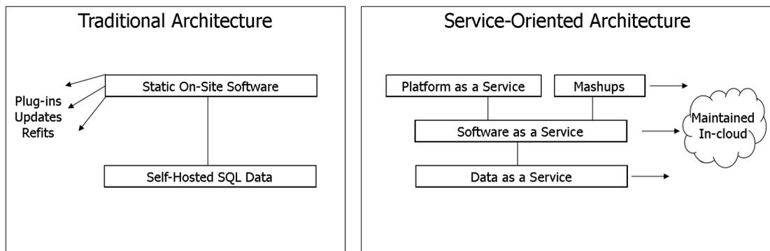
**Fig. 1.3** Comparison of traditional software architecture and SOA
