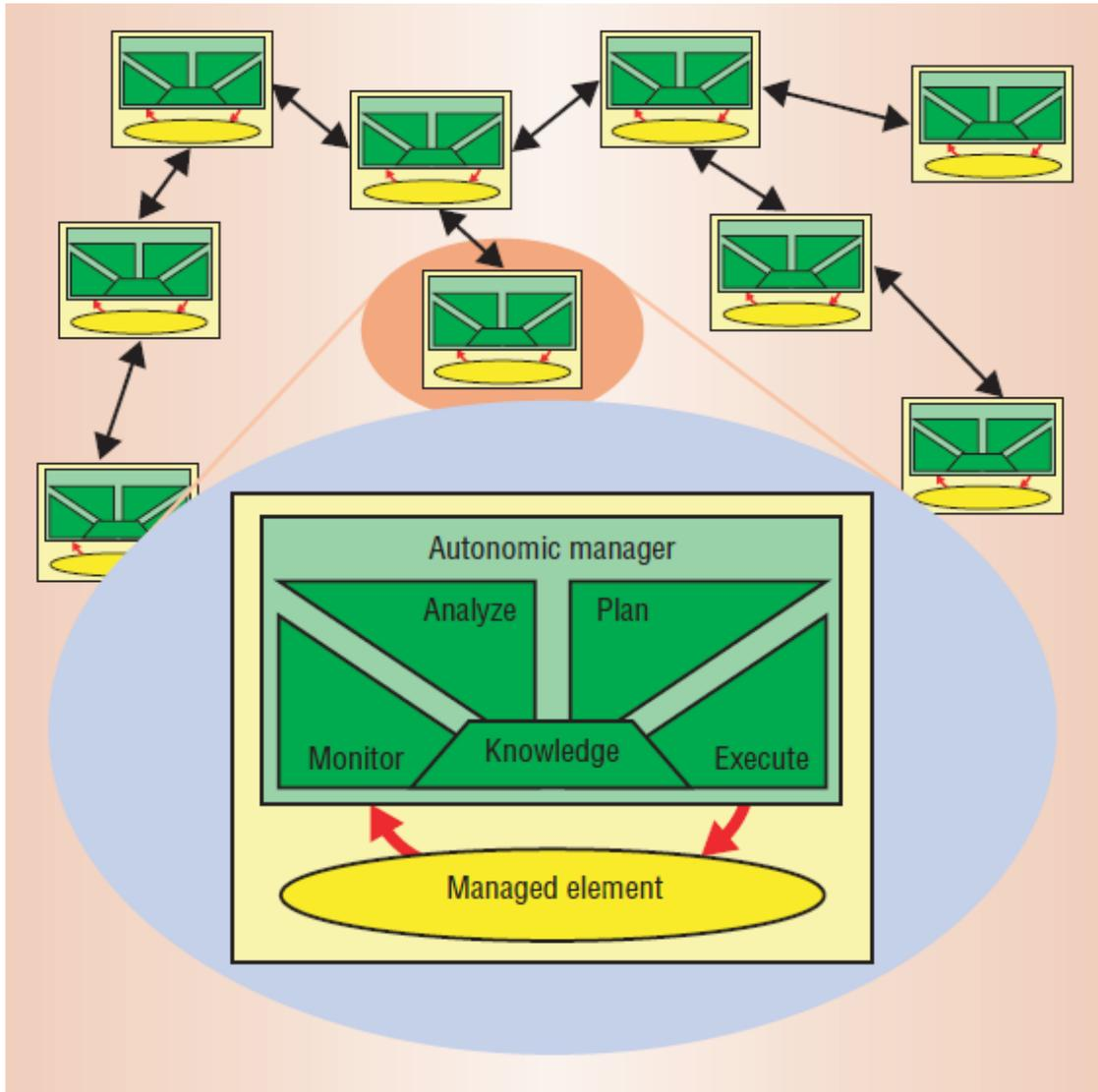
**Fig. 2.4** Structure of an autonomous element [Kephart & Chess, 2003]
