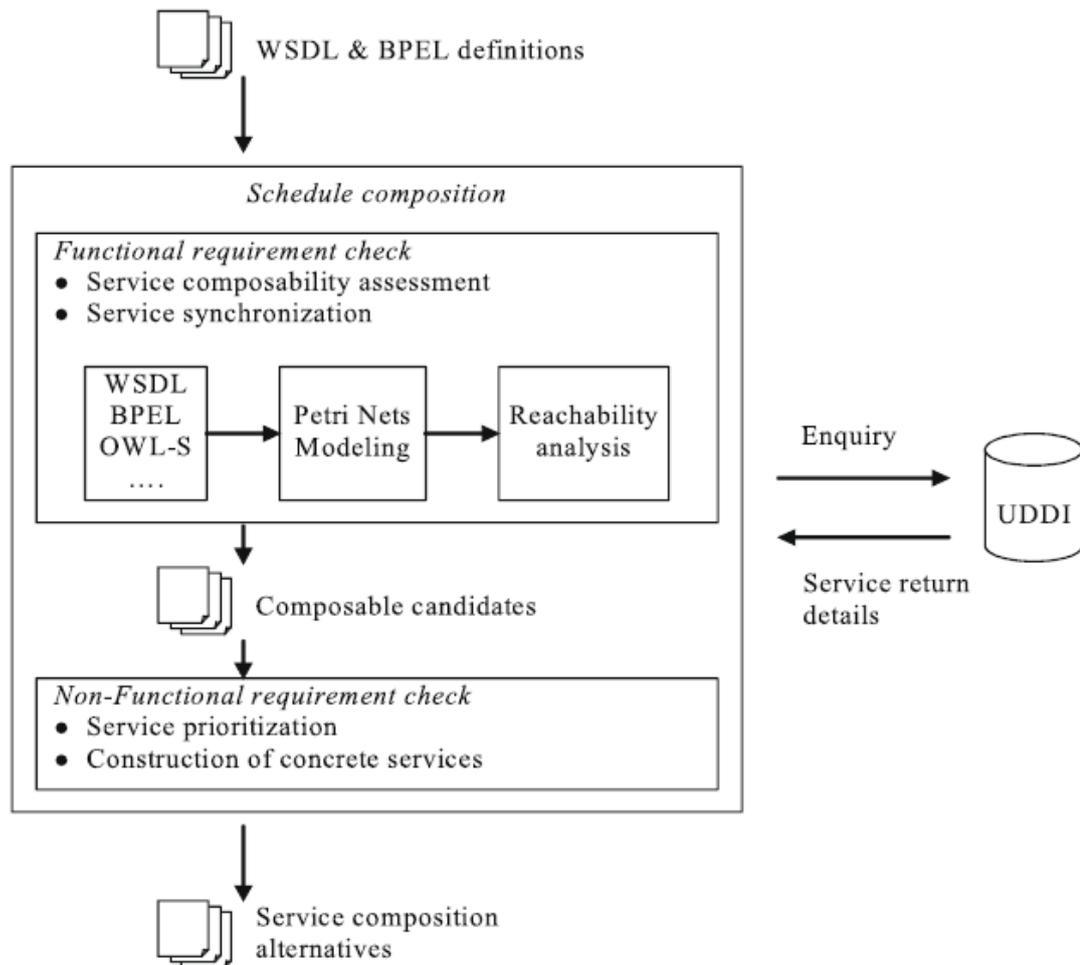
**Fig. 3.4** Functional validation methodology [Yoo et al, 2009]
