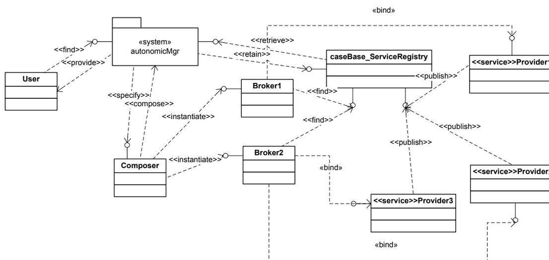
**Fig. 4.8** Meta model of the autonomous SOA in UML class diagram
