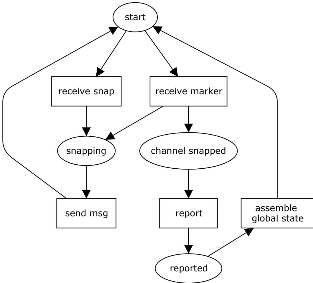
**Fig. 4.10** Petri Net model of the snapshot mechanism
