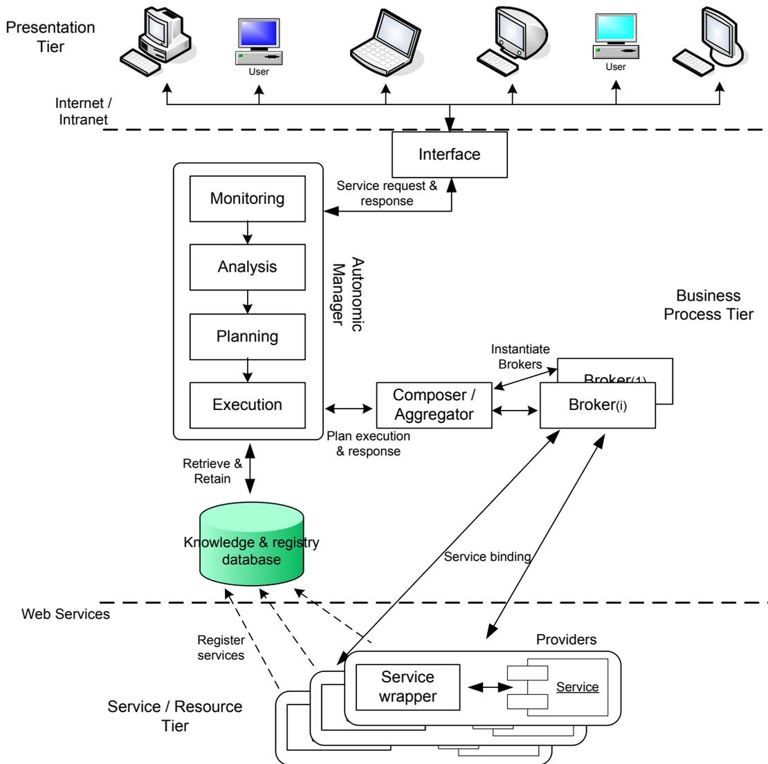
**Fig. 4.2** Overall architecture of the autonomic SOA
