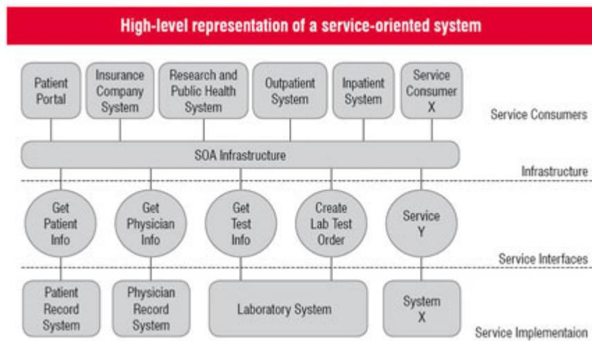
**Fig. 5.3** Example of SOA model in healthcare system [Smith & Lewis, 2009]
