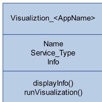
**Fig. 6.9** Visualization Service Provider class diagram
