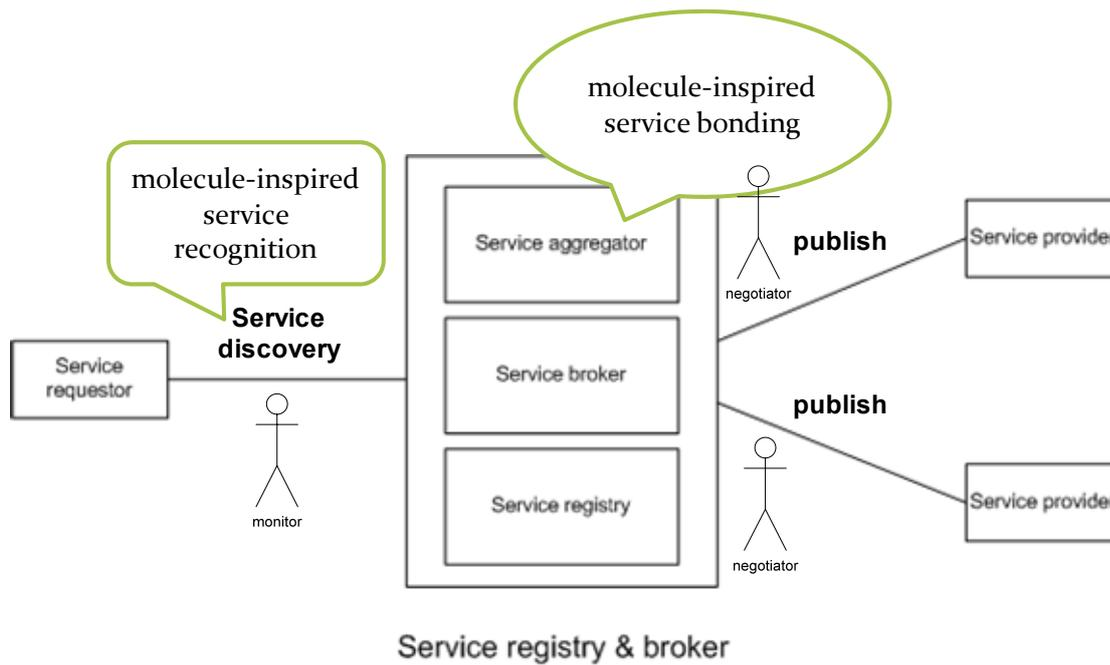
**Fig. 4.1** Initial service oriented architecture design
