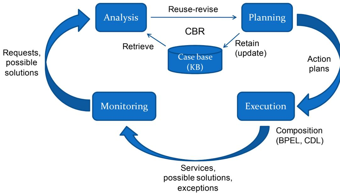
**Fig. 4.5** Adaptation of autonomic cycle and CBR in autonomic SOA
