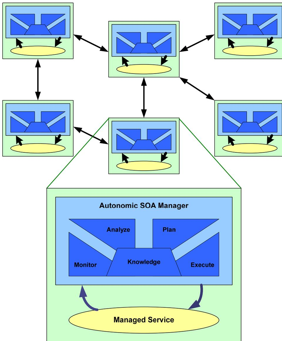
Fig. 3.3 Structure of autonomous SOA (adapted from [Kephart & Chess, 2003])
