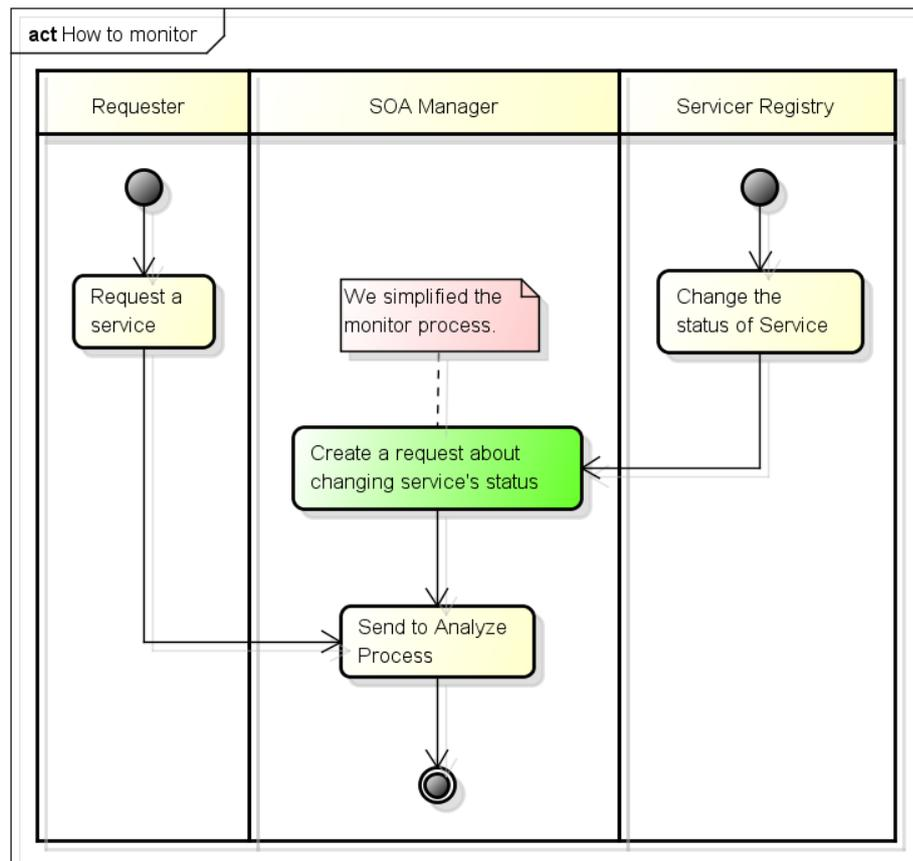
**Fig. 4.3** Monitoring process
