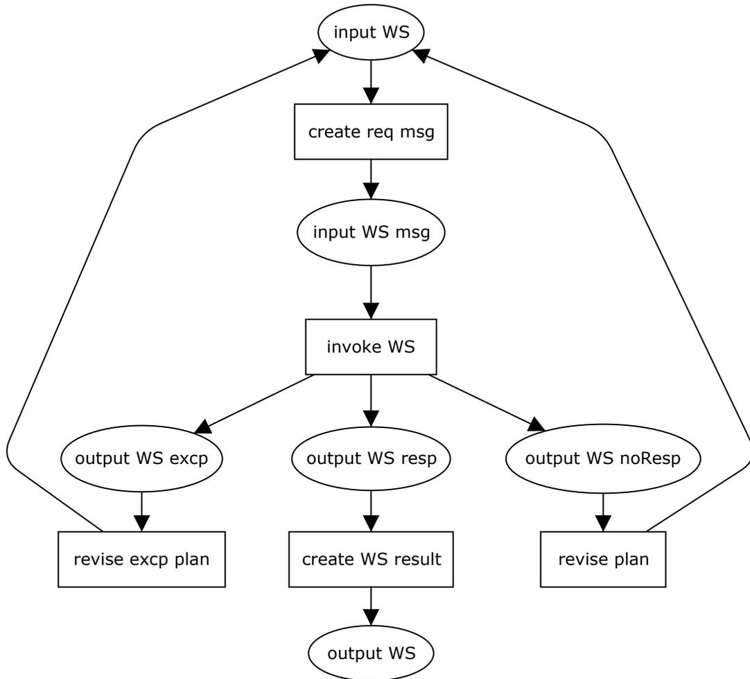
**Fig. 4.13** Petri Net model of the invoke operation
