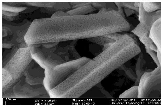
Figure 29: Image of zinc oxide sintered for 2 hours magnified at 50k
