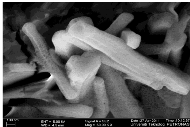
Figure 28: Image of zinc oxide sintered for 1 hour magnified at 50k
