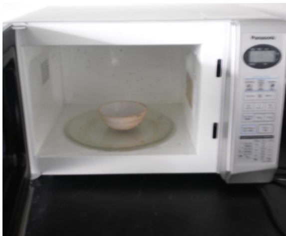
Figure 12: Sintering using Microwave
