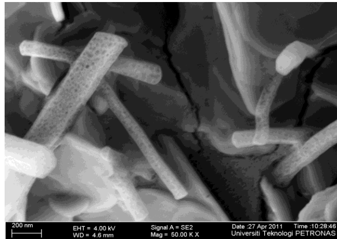
Figure 30: Image of zinc oxide sintered for 3 hours magnified at 50k
