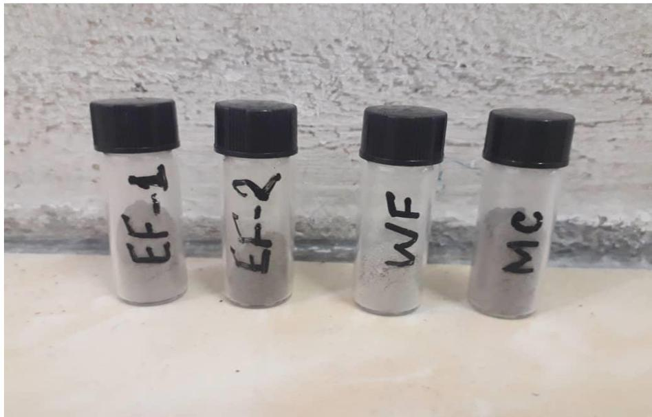
Figure 3.2: Shale samples from Eagle ford, Mancos, and Wolfcamp formation in powder form
