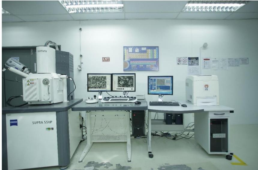
Figure 3.5: Field emission scanning electron microscopy (SUPRA 55VP)
