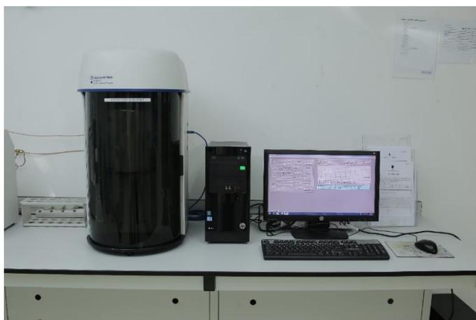
Figure 3.9: Surface area analyzer and porosimetry system
