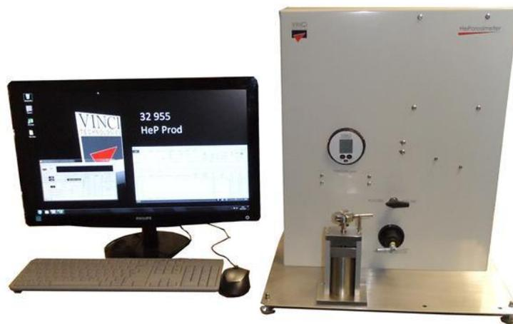
Figure 3.11: Helium Porosimeter
