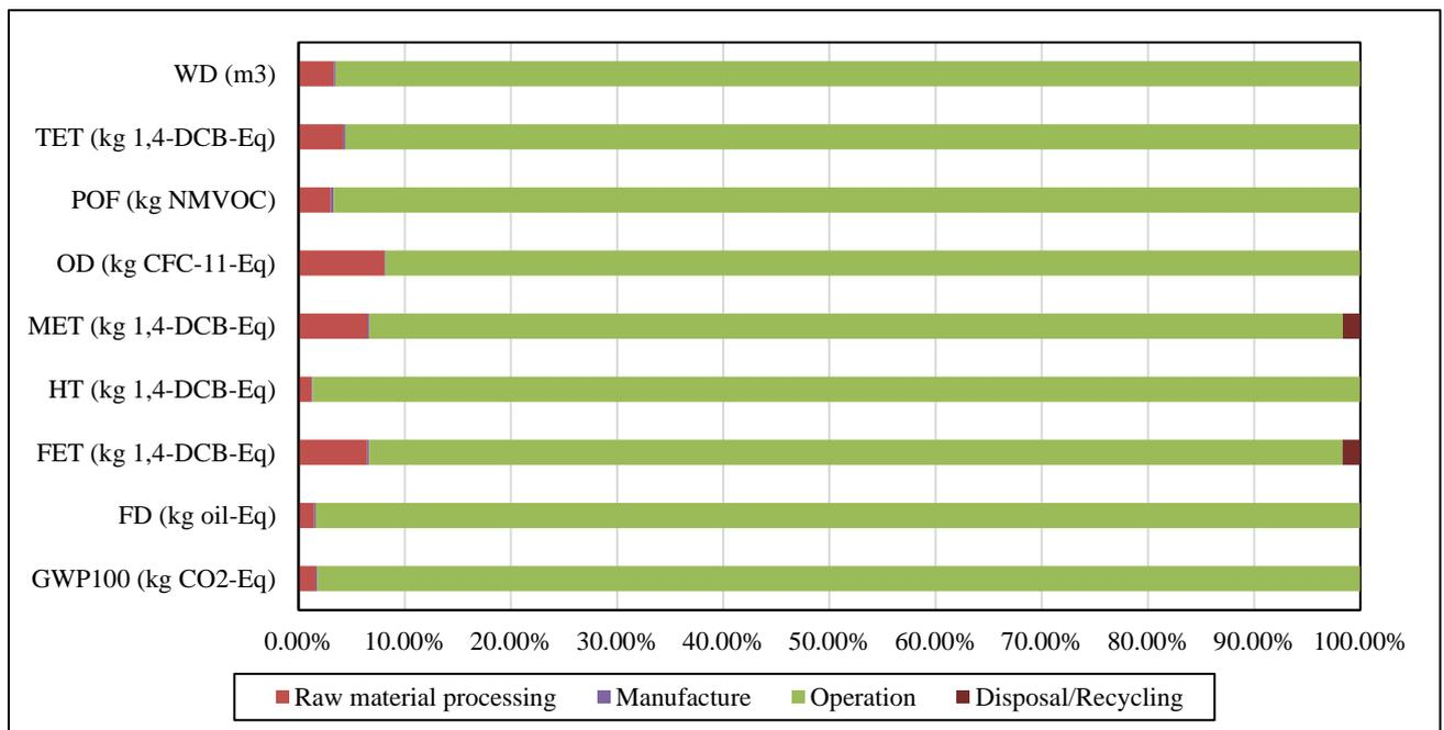
Figure 4.6: Contribution of different life cycle stages of the VCS to the life cycle impacts categories.
