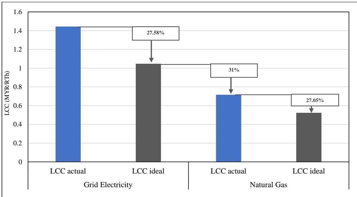
Figure 4.10: LCC/RTh results of the VCC systems under the considered scenarios.
