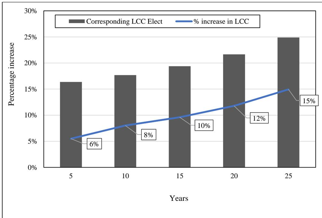
Figure 4.14: **Percentage increase in LCC using commercial grid electricity as an energy source.**
