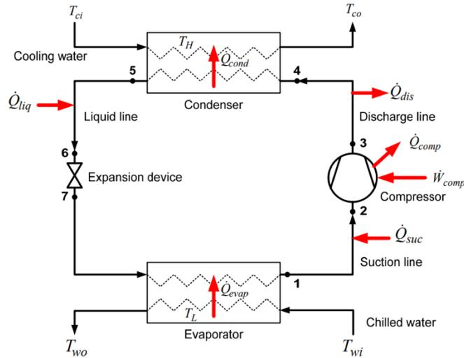
Figure 2.1: **Schematic diagram of a vapor-compression system [20].**
