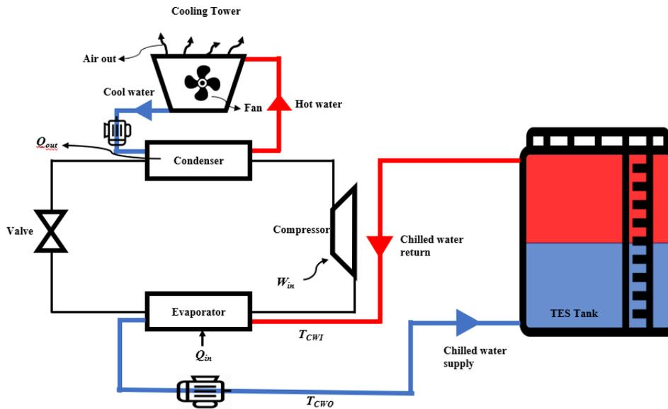
Figure 3.2: Schematic diagram of a Vapor-Compression System.
