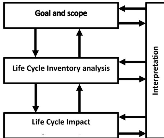
Figure 2.3: LCA Framework ISO 14040 [35]
