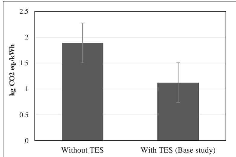
Figure 4.7: **The carbon footprint of a VCC system installed with and without a TES tank.**
