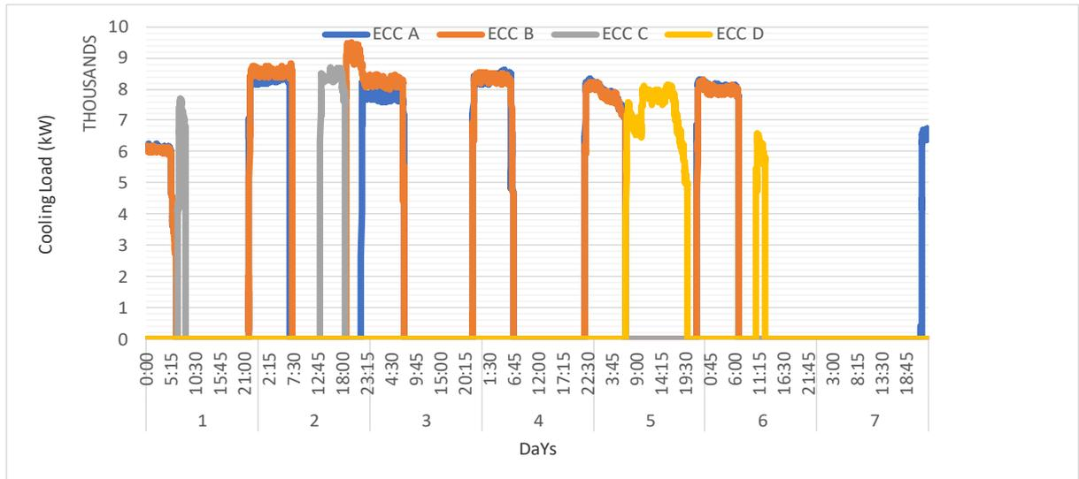
Figure 3.10: A week operation of the four VCC systems.
