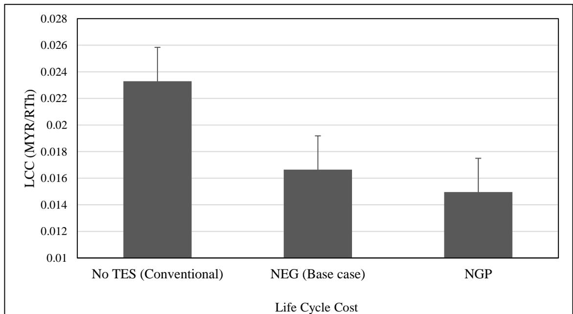
**Figure 4.9: LCC per refrigeration of the VCS systems using electricity and natural gas as energy sources.**
