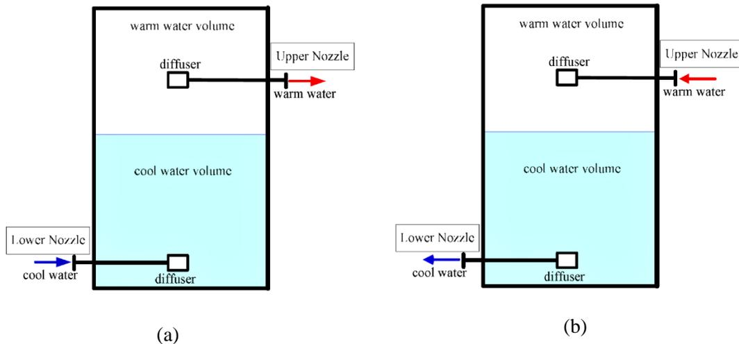
Figure 2.2: **Charging and discharging cycle of the TES tank: (a) Charging: (b) Discharging**
