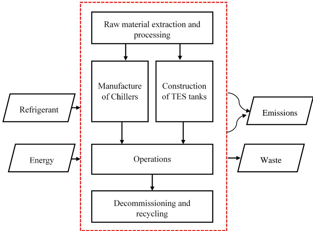
Figure 3.11: **System boundary of the LCA study**
