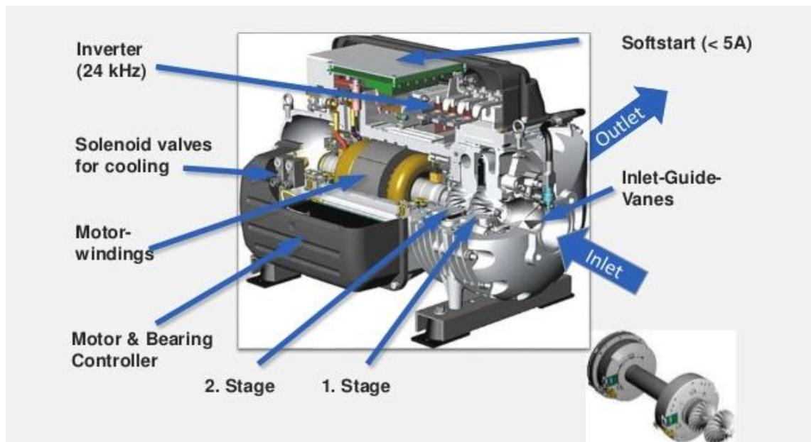
Figure 3.14: **Parts of the Danfoss Turbocor centrifugal chiller [77]**
