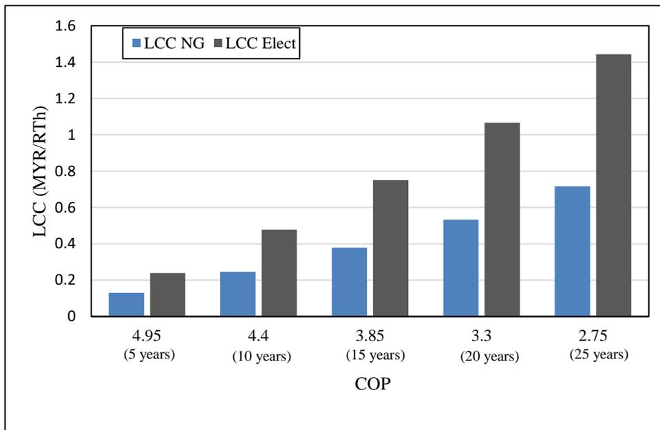
**Figure 4.13: Cost per refrigeration result of the VCS system through its lifespan for both scenarios.**
