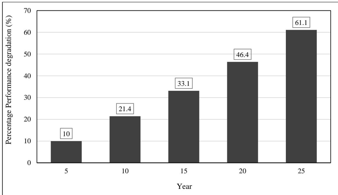
**Figure 4.4: Percentage performance degradation of the VCC system throughout its lifetime.**
