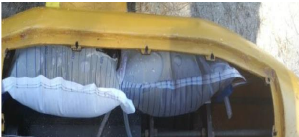
Figure A.3: Setup roll control module with water bladder in proposed design
