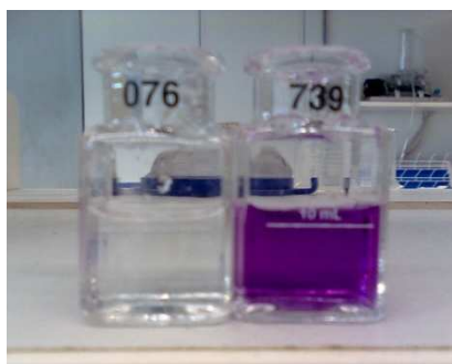
Figure B: CuVer 1 Copper Reagent Powder Pillows dissolved in \text{Cu}^{2+} solution (purple solution) before being tested using UV-vis spectrophotometer
