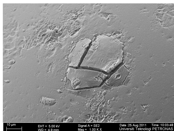
Figure A: Surface comparison between fresh resin (top), resin after pretreatment (middle) and resin after treatment with \text{Cu}^{2+} .
