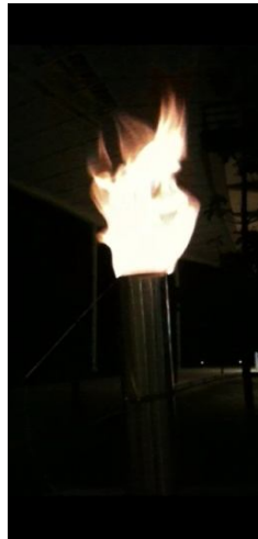
Figure 4.5: Flare produced from sugarcane bagasse gasification
