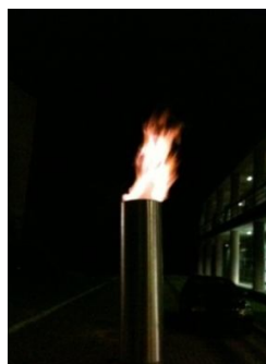
Figure 4.3: Flare produced from OPF gasification
