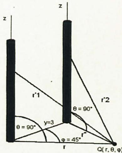
Figure 4.1 The position of the wires in Spherical coordinates
