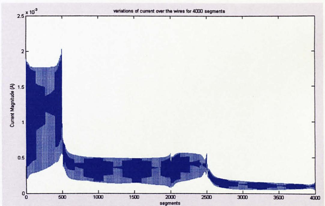
Figure 4.10 The standing wave on the wires before terminating the model by 13 Ohm resistance
