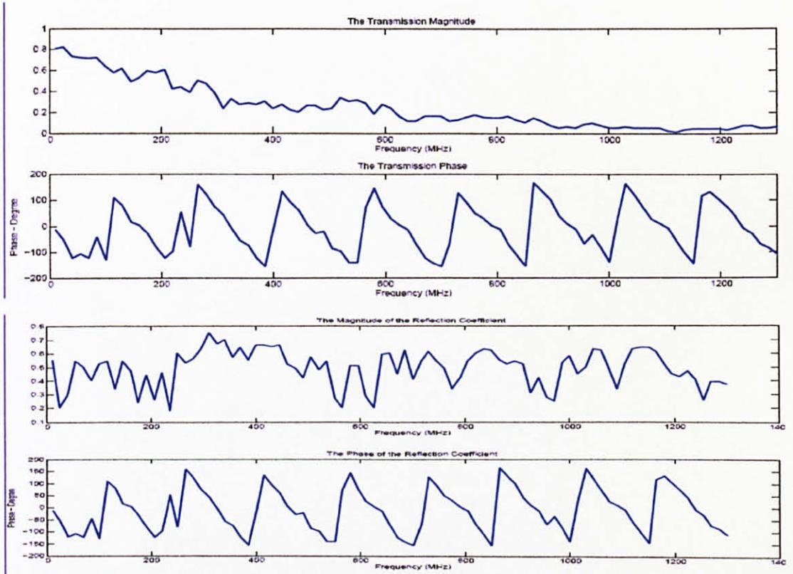
Figure 4.16 The Transmission and Reflection magnitude and phase of the transmission line, obtained from the circuit analyzer
