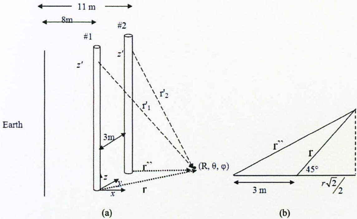
Figure 4.3 (a) The distances from the wires to the desired point, (b) Reflection with the distance
