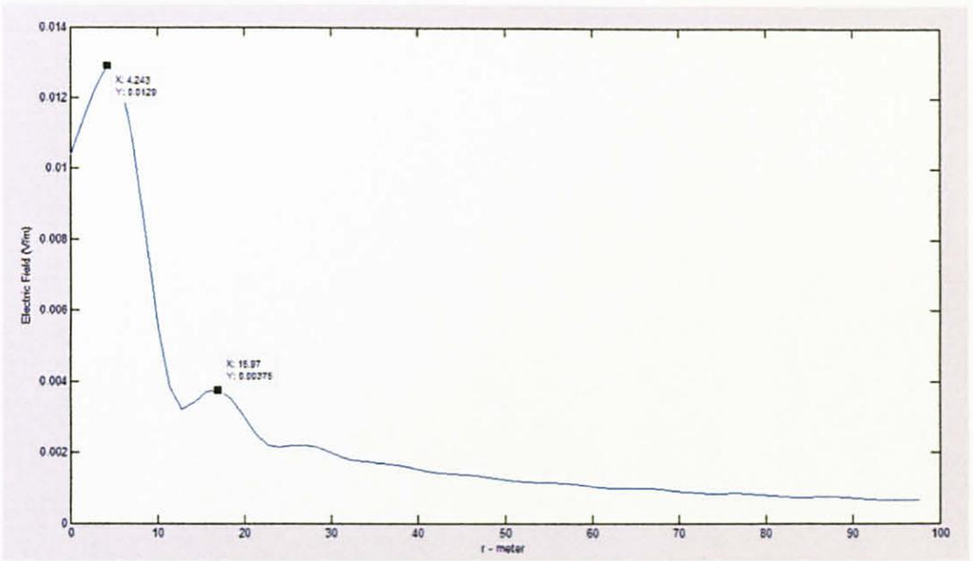
Figure 4.8 The electric field in free space obtained in NEC WIN Professional software
