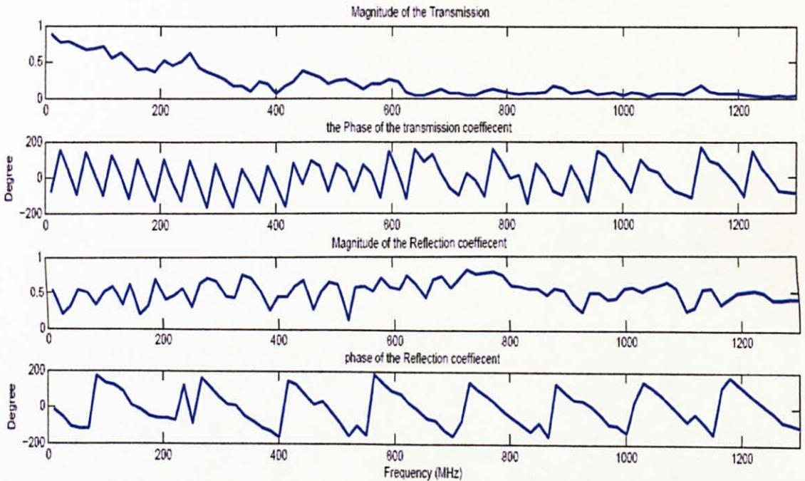
Figure 4.14 The Transmission and Reflection magnitude and phase of the transmission line, obtained from the circuit analyzer
