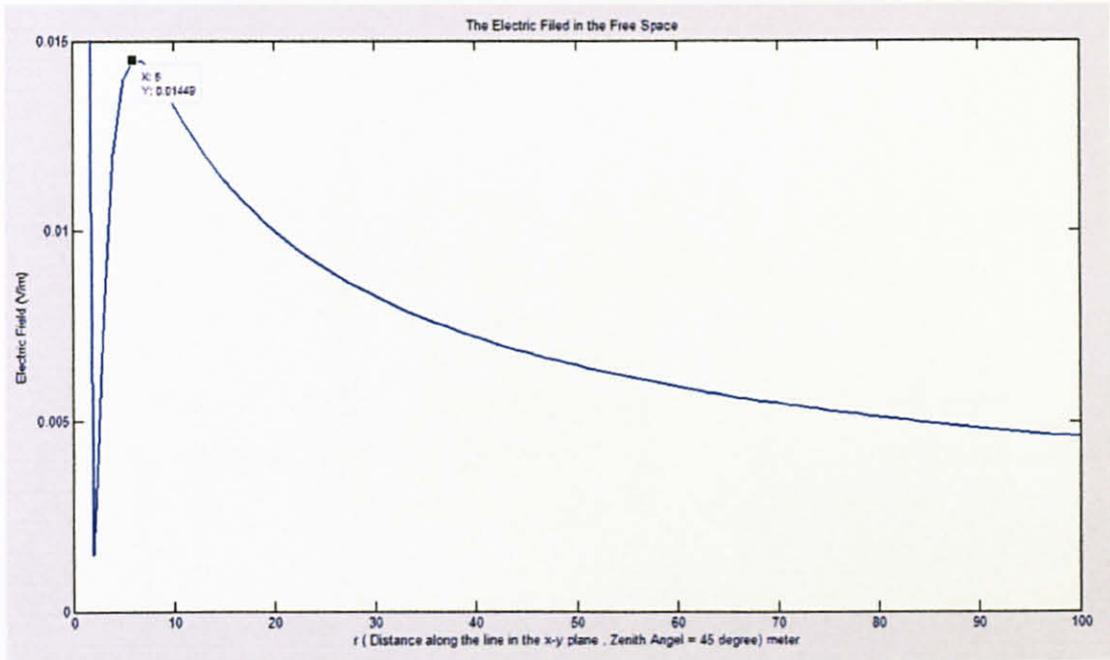
Figure 4.6 The electric field in free space obtained from codes implemented in MATLAB
