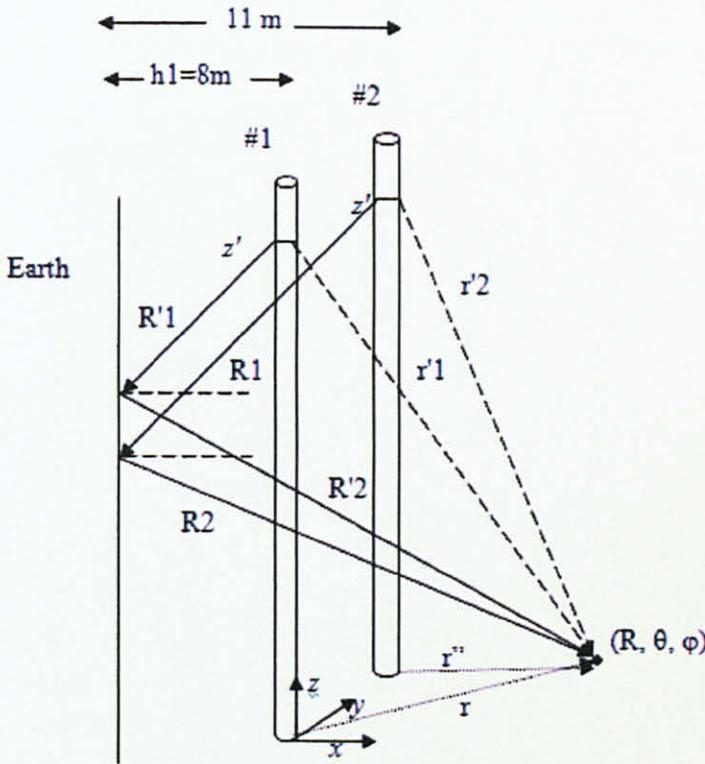
Figure 4.2 The reflected distance for the two wires
