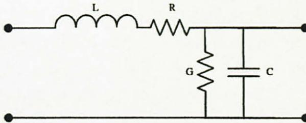
Figure 2.3 The equivalent circuit of a two conductor transmission line
