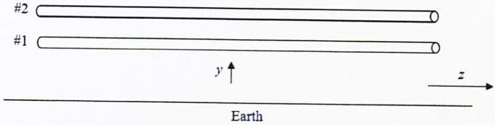
Figure 2.4 The BPL system, consisting of the two vertically displaced wires suspended over the earth
