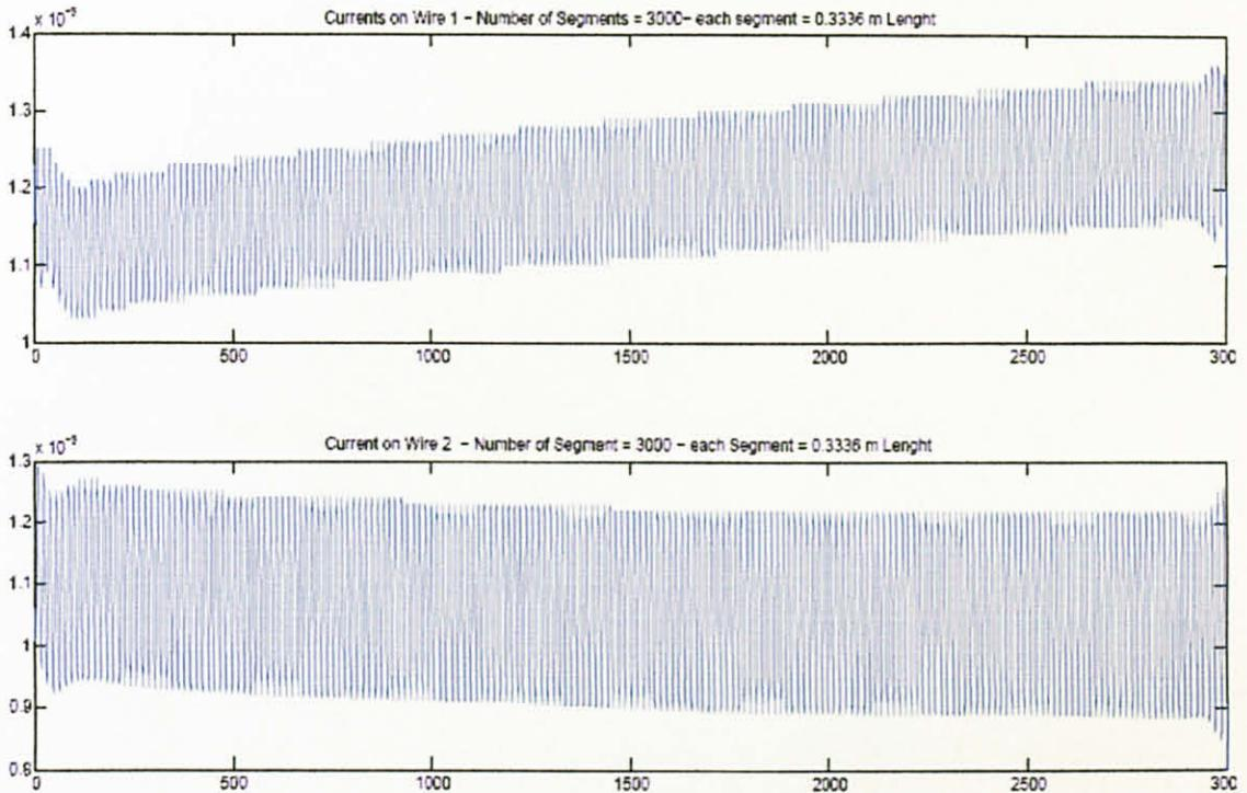
Figure 4.11 the current on the both wires after eliminating the standing waves
