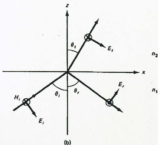
Figure 2.6 The reflection on a plane wave incident on a single boundary separating the two media (a) Perpendicular and (b) Parallel Polarization
