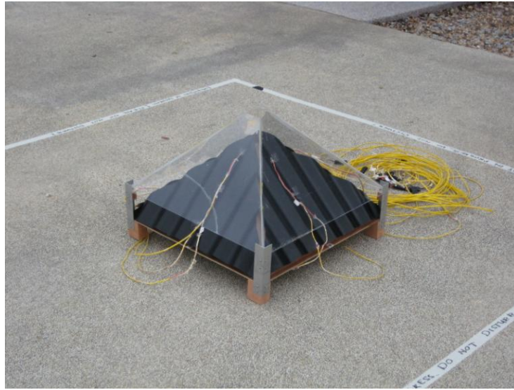
Fig. 3.1 Image of the placement of the thermocouples on the surface of the collector
