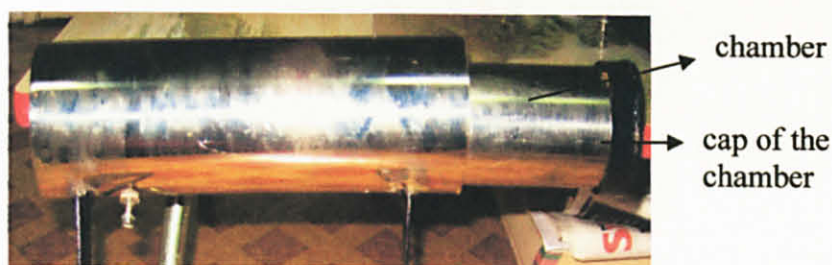
Figure 21: Chamber of Microreactor
