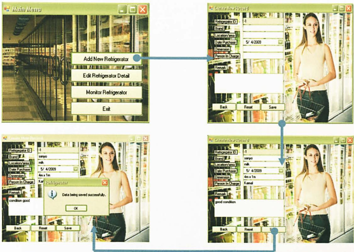
Figure 14: Add New Refrigerator Interface
