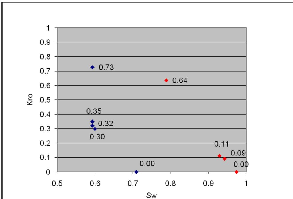
Figure 9: Saturation of water VS. Relative Permeability of Oil Curve
