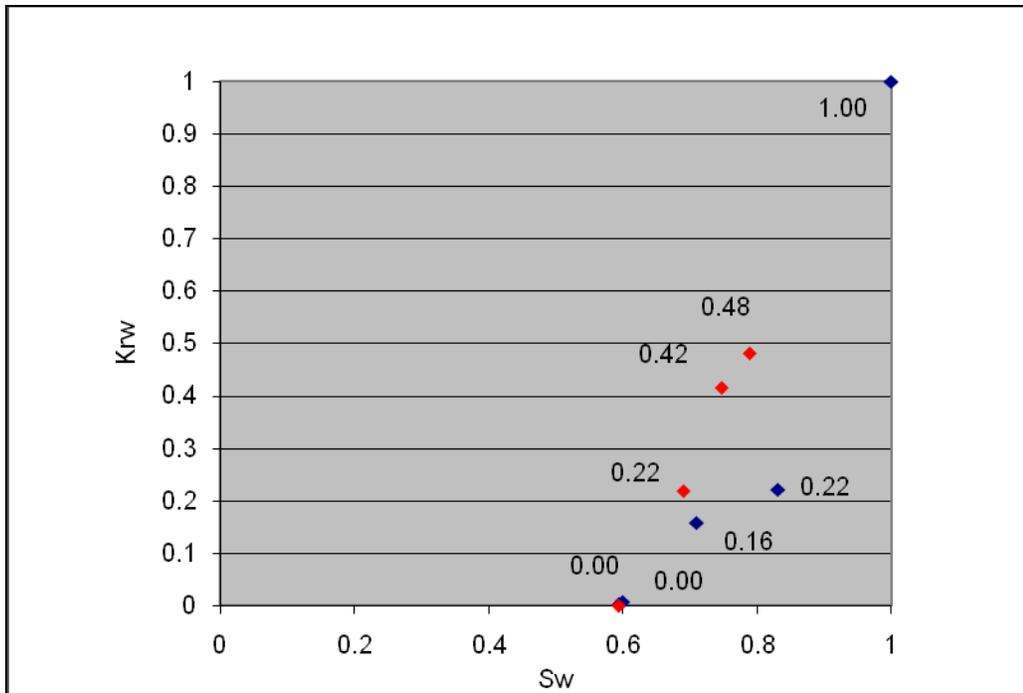
Figure 8: Saturation of water VS. Relative Permeability of water Curve
