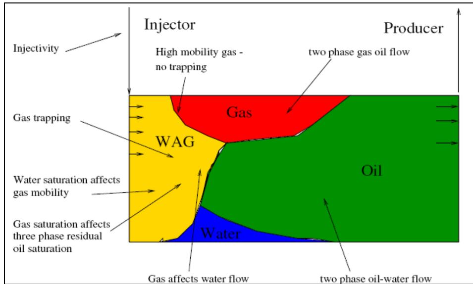
Figure 1: Principal Drawing of a WAG displacement and schematic outline of multiphase flow mechanics
