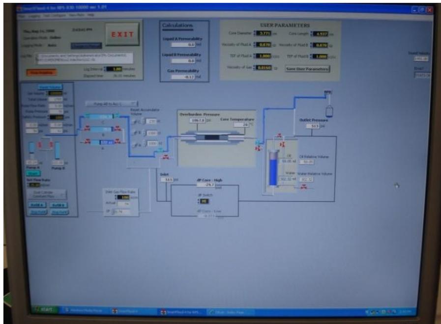
Figure 6: SmartFlood Software for Relative PermeabilityMachine
